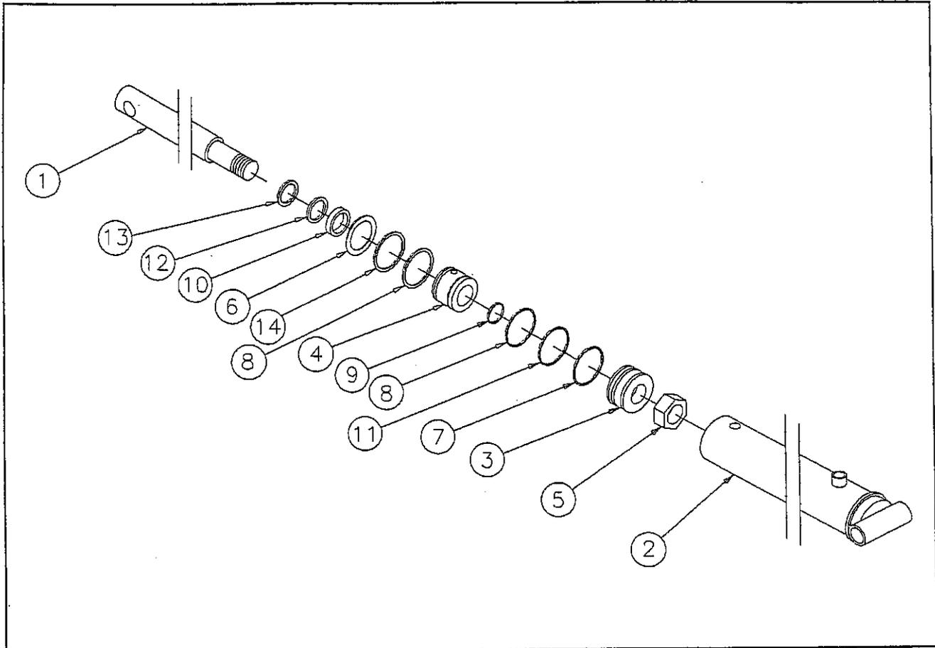
Figure 6-8 Pintle Hitch Trailer Tilt Cylinder Assembly
