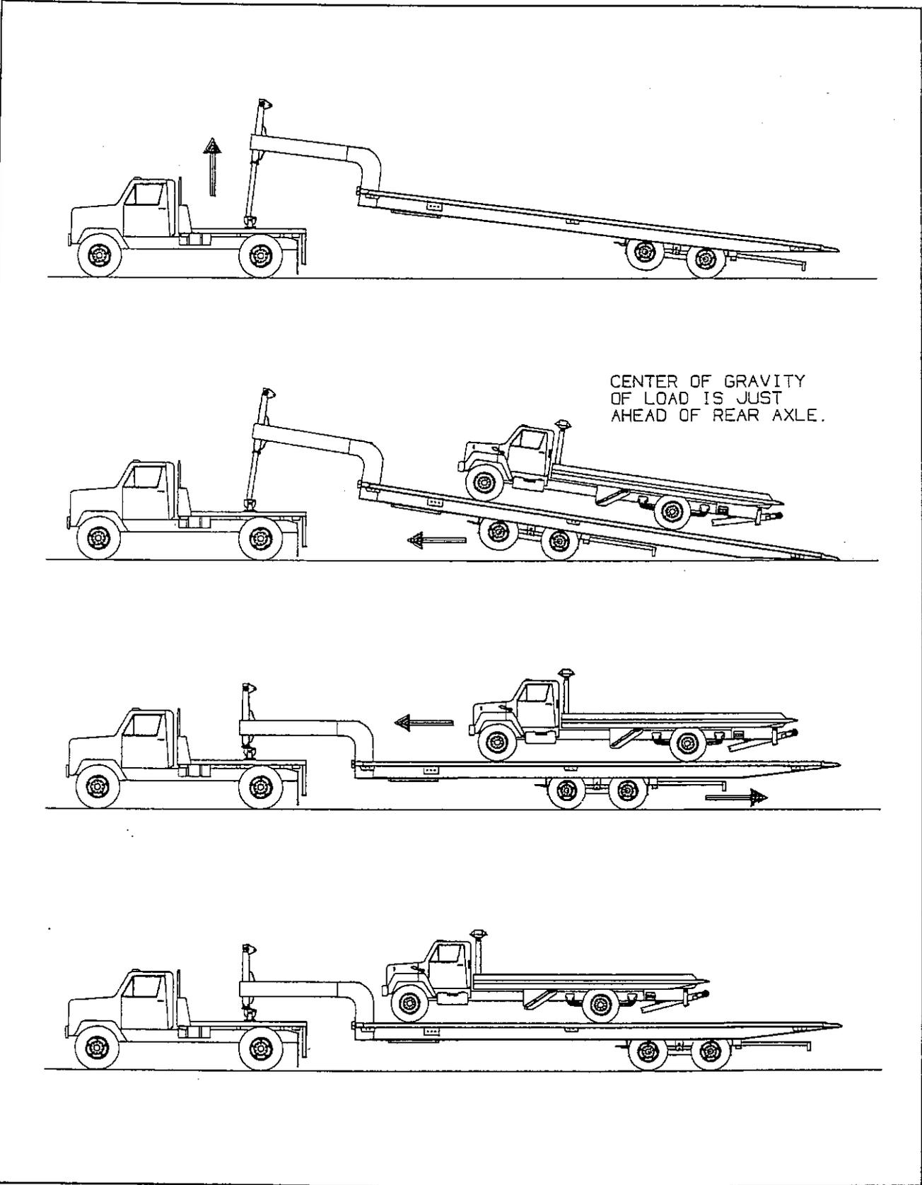
Figure 3-3 Steps for Loading and Unloading
