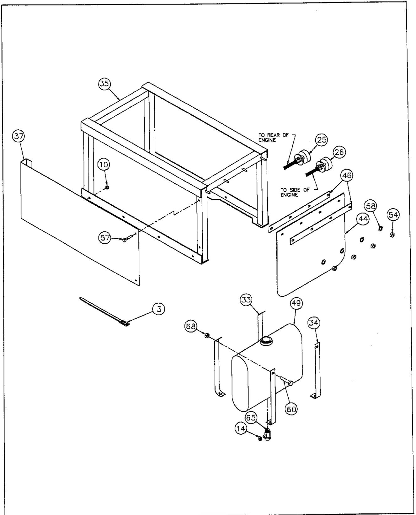
Figure 6-27 Auxiliary Engine Package (2 of 2)
