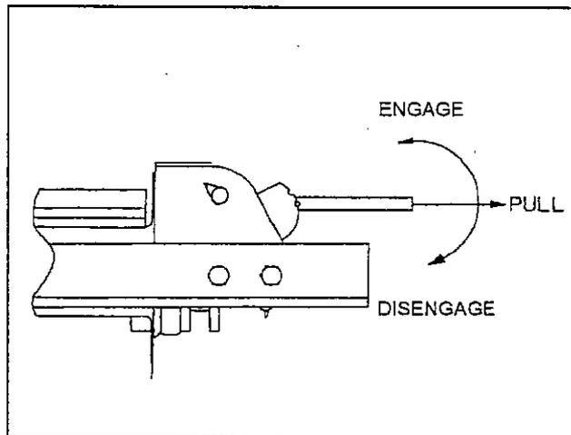
Figure 3-5 12,000# Winch Clutch
