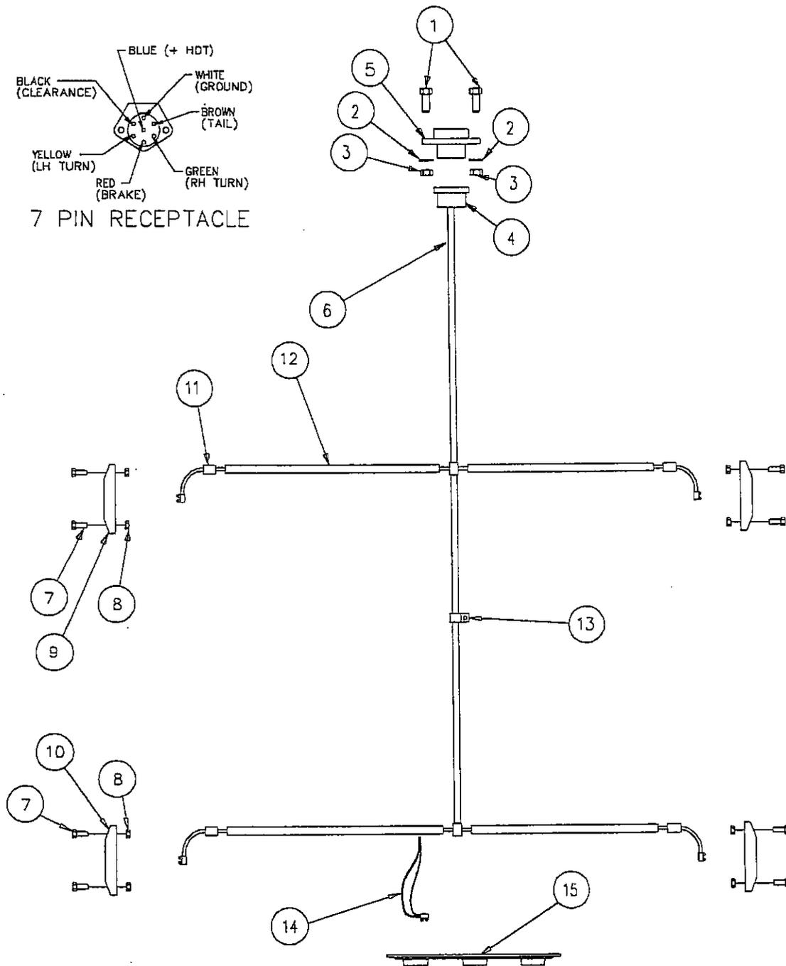
Figure 6-29 Truck Bed Electrical System
