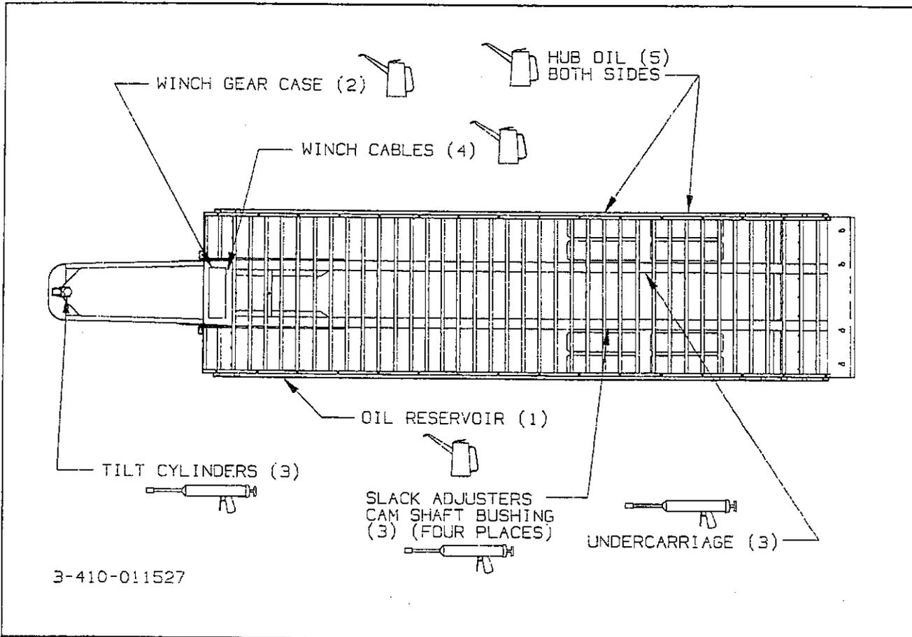
Figure 4-1 Lubrication Points
