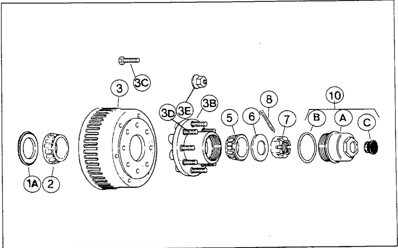
Figure 6-19 Hub and Drum Assembly
