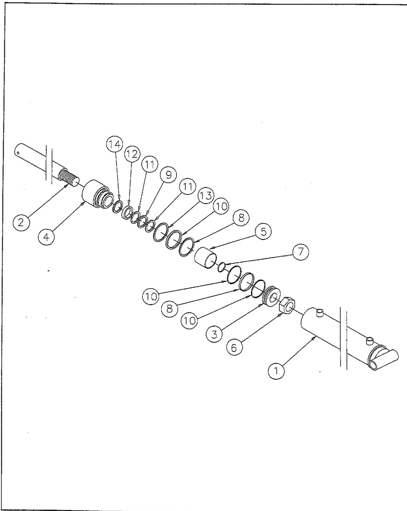
Figure 6-9 Undercarriage Slide Cylinder Assembly
