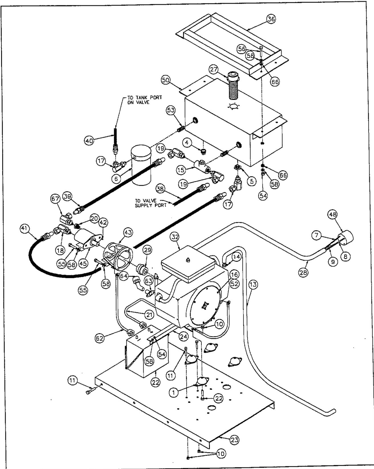
Figure 6-26 Auxiliary Engine Package (1 of 2)
