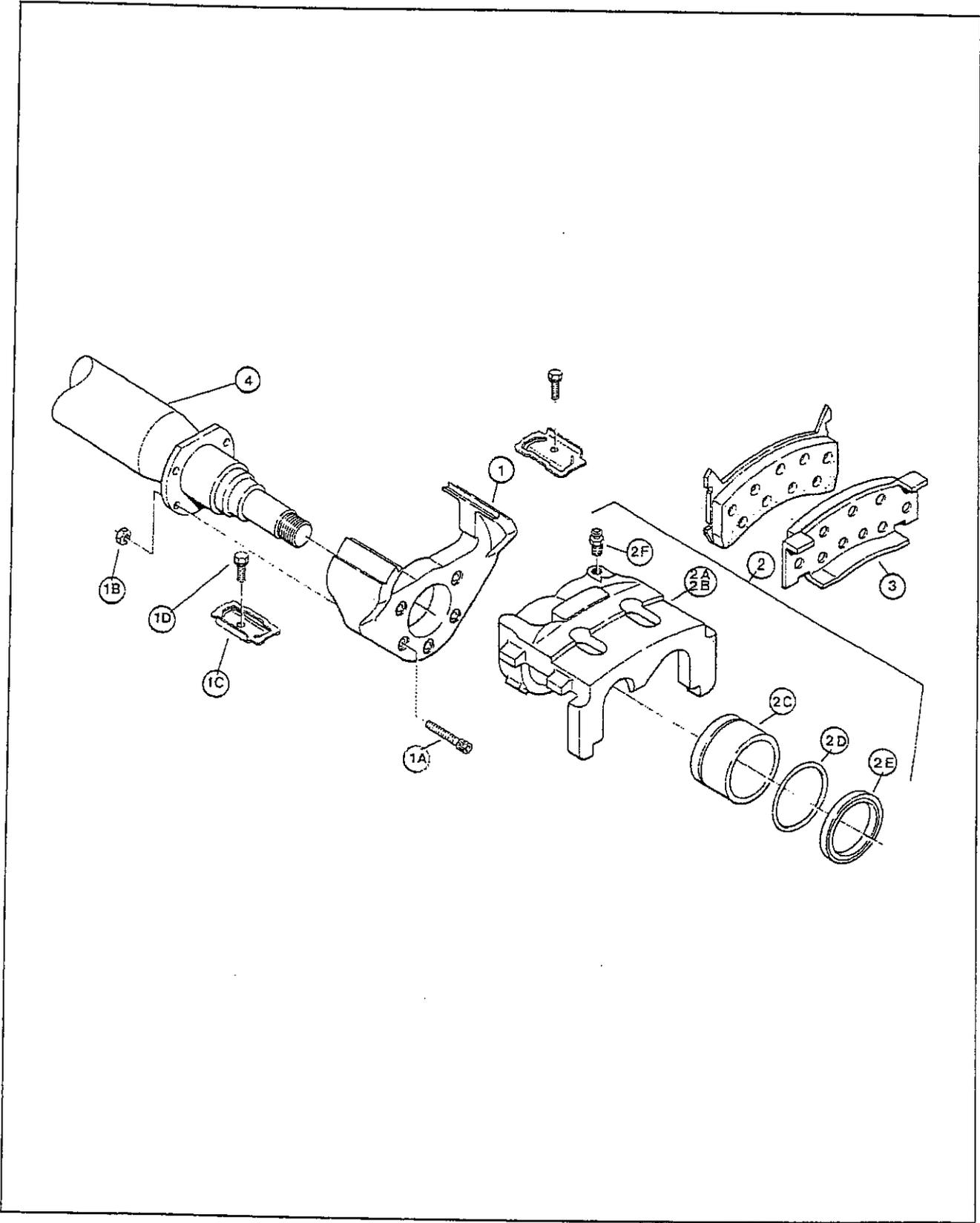
Figure 6-13 Hydraulic Disc Brake and Axle Assembly
