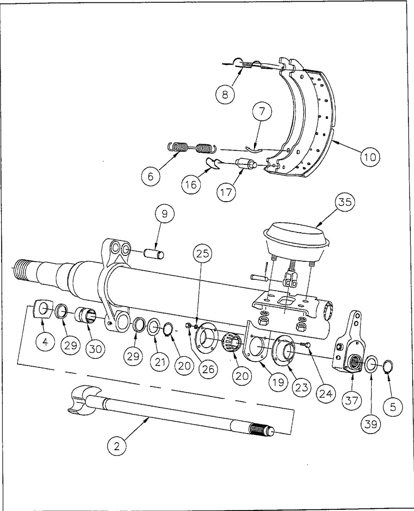
Figure 6-14 Air Brake and Axle Assembly
