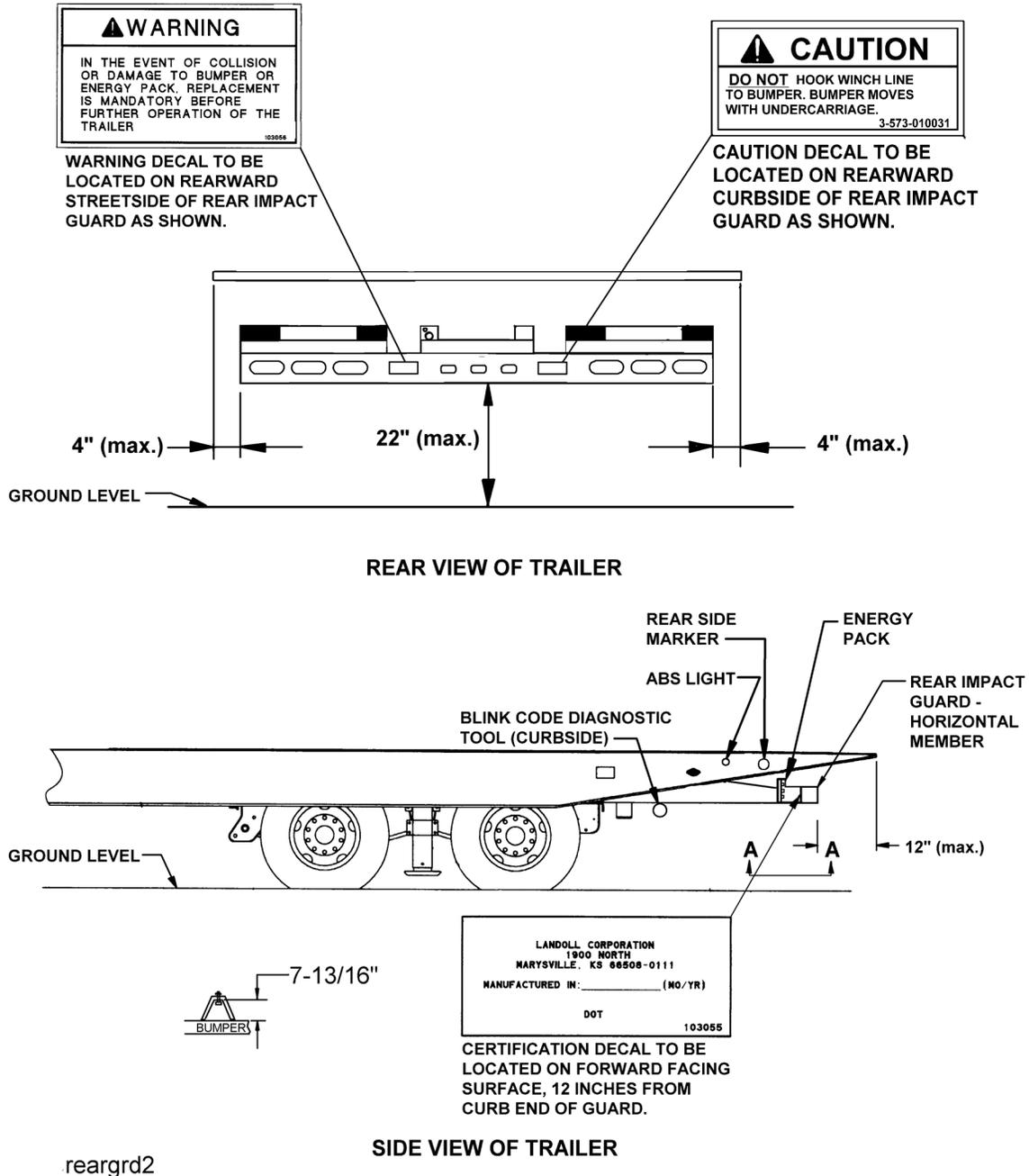
**Figure 3-14: Rear Impact Guard and Anti-Lock Brake System**
