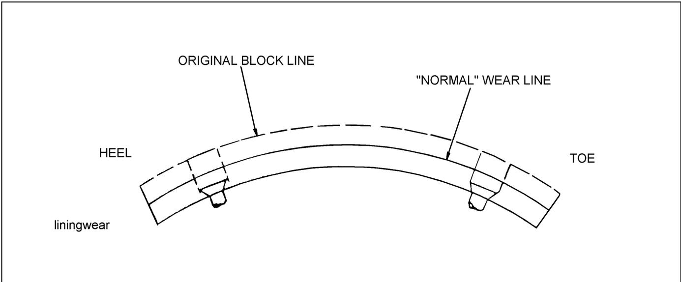
Figure 4-10: Brake Lining Wear
