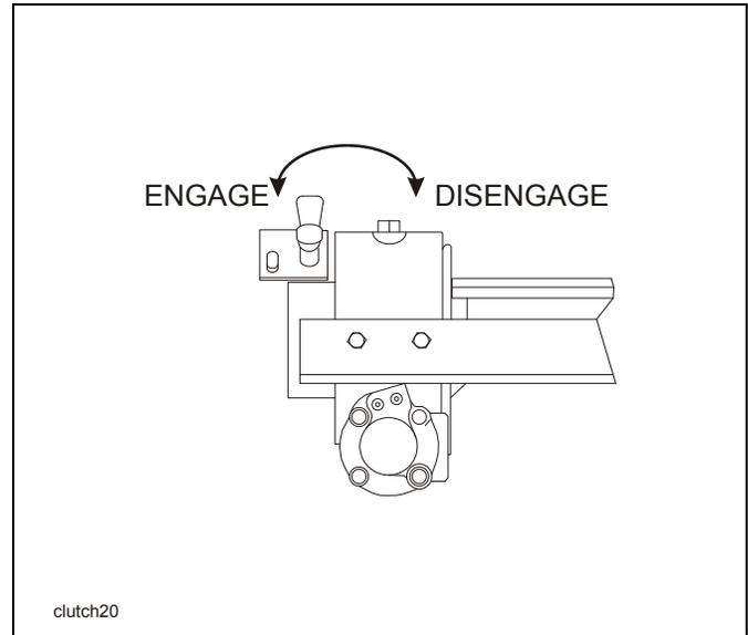
**Figure 3-9: 20,000# Winch Manual Clutch**
