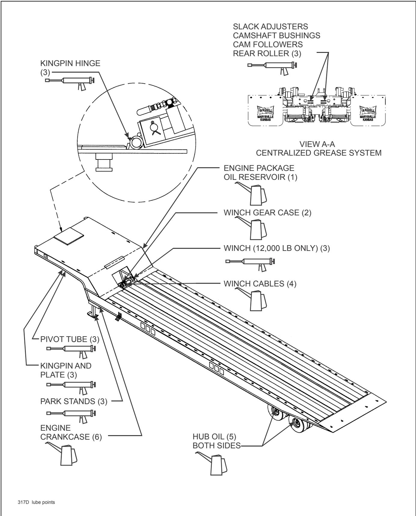
**Figure 4-1: Lubrication Points**
