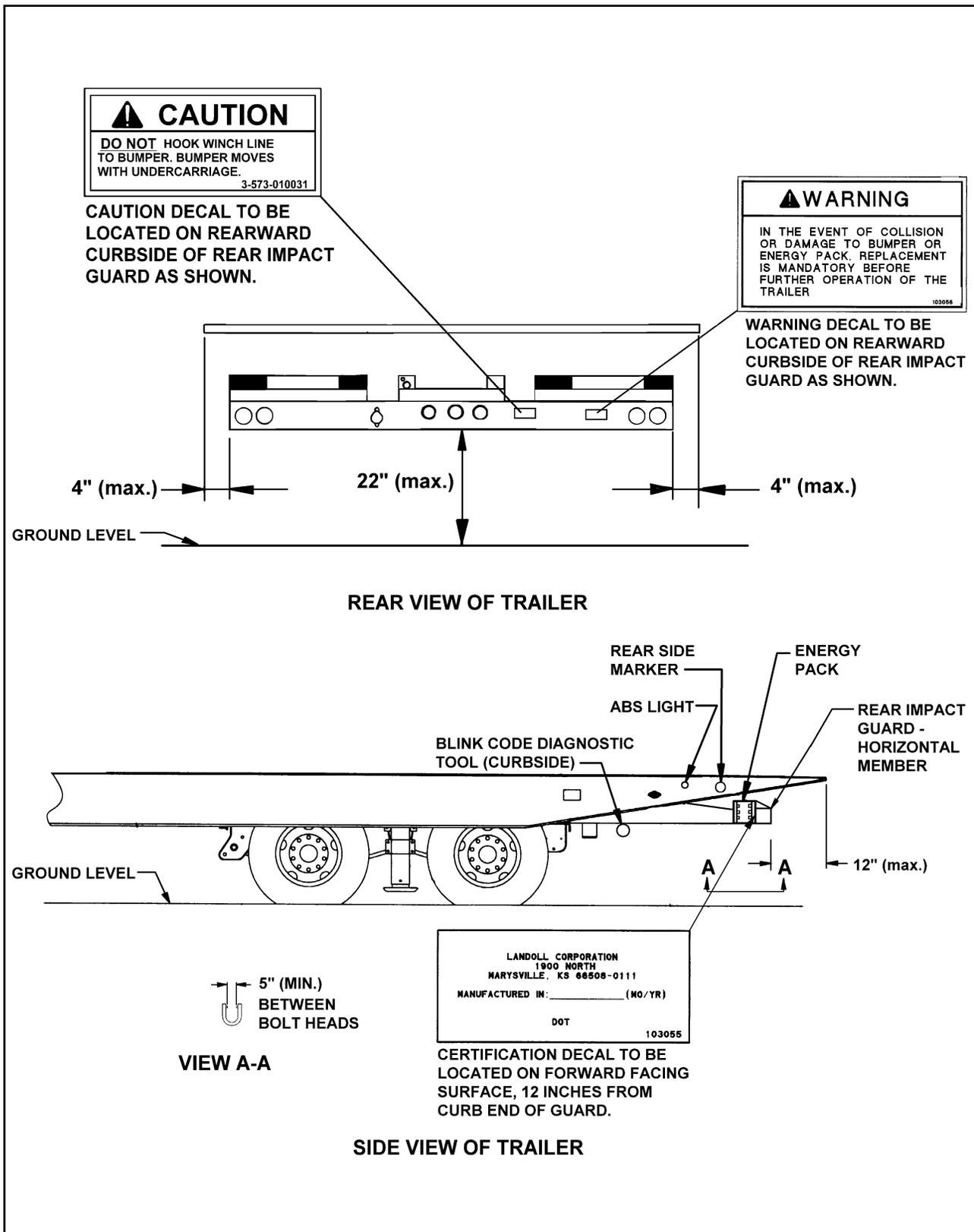
Figure 3-7 Rear Impact Guard System
