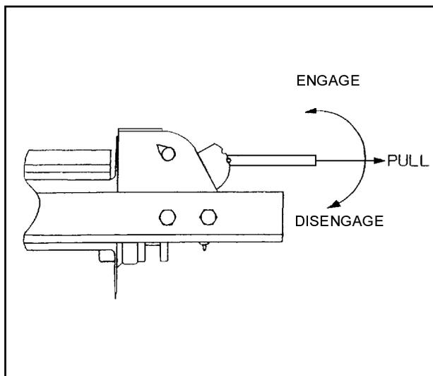
**Figure 3-4 12,000# Winch Clutch**
