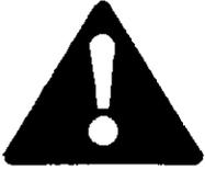
THIS IS THE INTERNATIONAL SAFETY ALERT SYMBOL. IT ALERTS THE OPERATOR TO IMPORTANT SAFETY MESSAGES ON THE MACHINE AND IN THIS MANUAL. CAREFULLY READ AND STUDY THESE LABELS AND MESSAGES BEFORE MACHINE ASSEMBLY AND OPERATION. THERE ARE THREE TYPES OF SAFETY ALERT MESSAGES:
