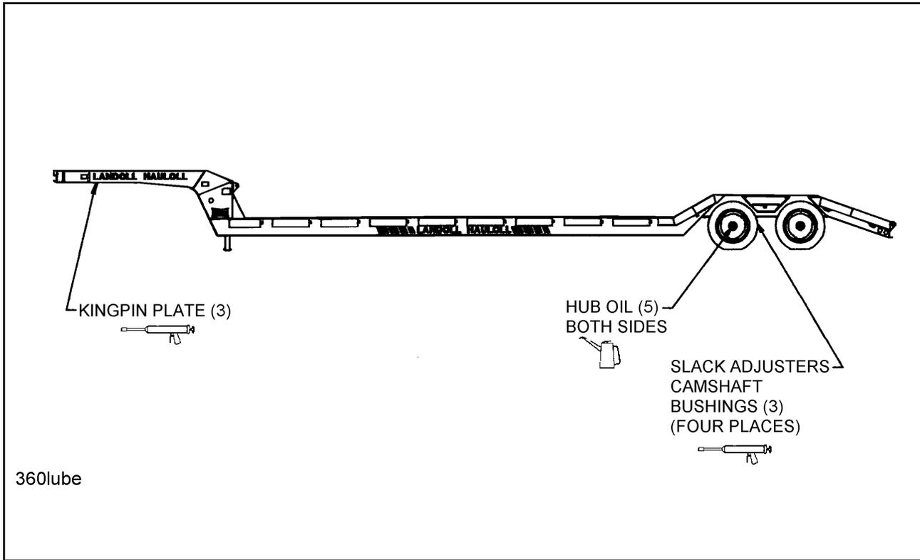
Figure 4-1 Lubrication Points
