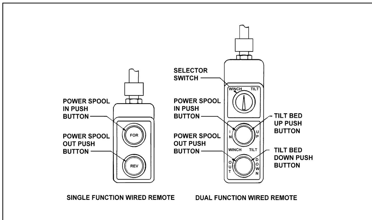
Figure 3-6 Examples of Remote Control Options
