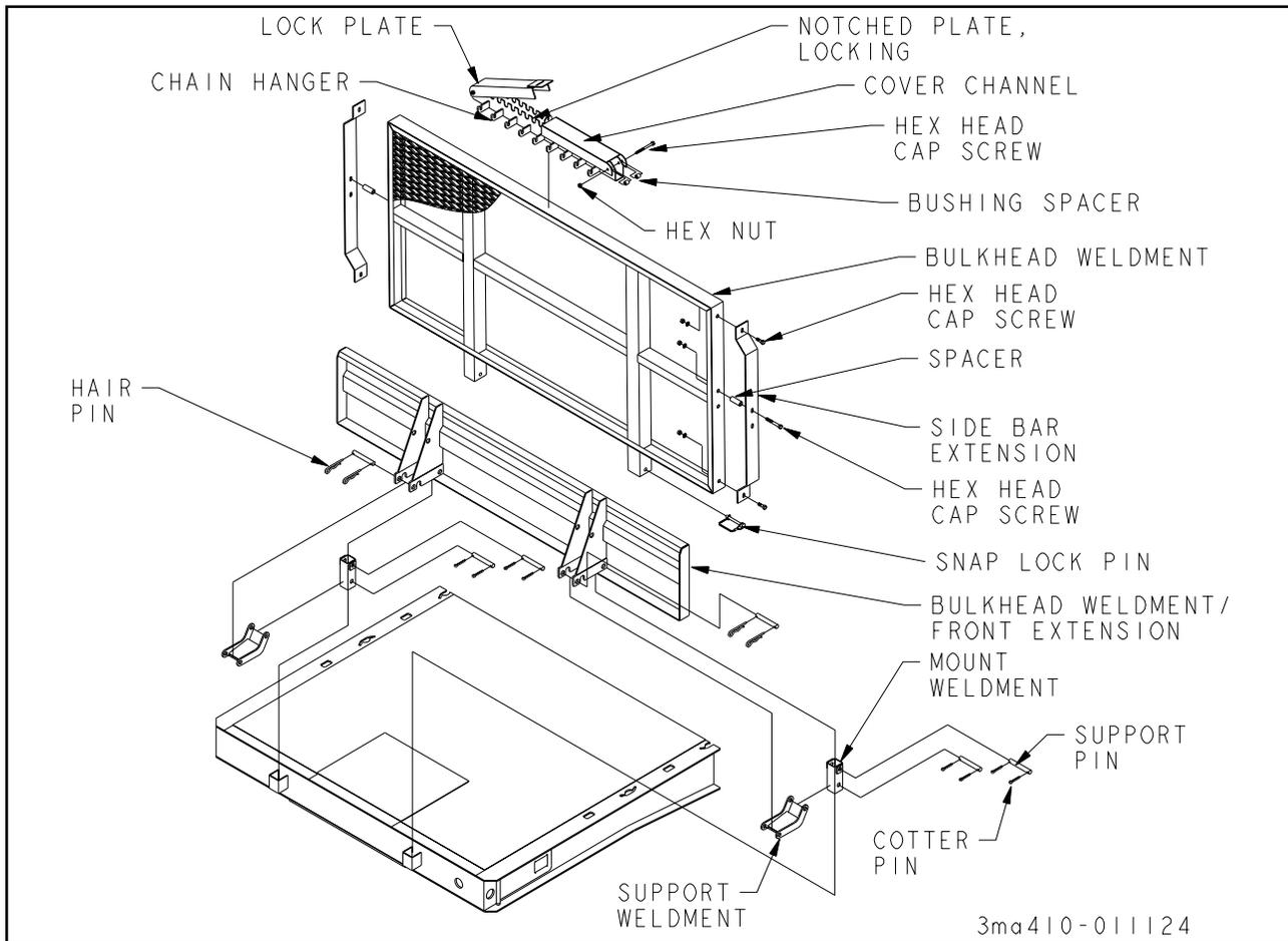
**Figure 3-5 Front Extension/Bulkhead**
