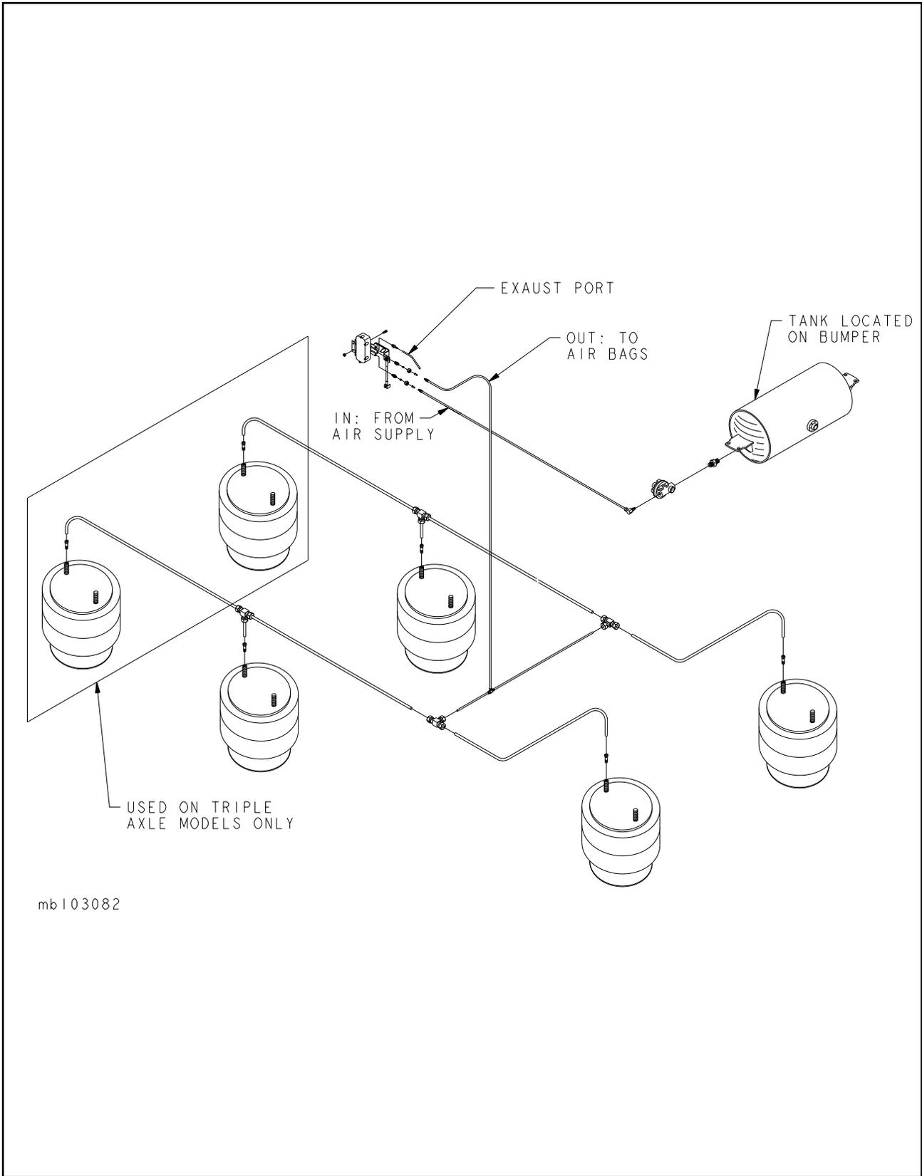
**Figure 4-4 Tandem Axle Air Ride Suspension System**
