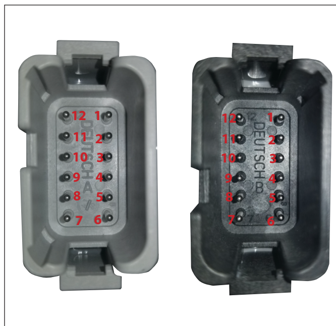
Figure 3-16: Deutsch A and B Pin locations
