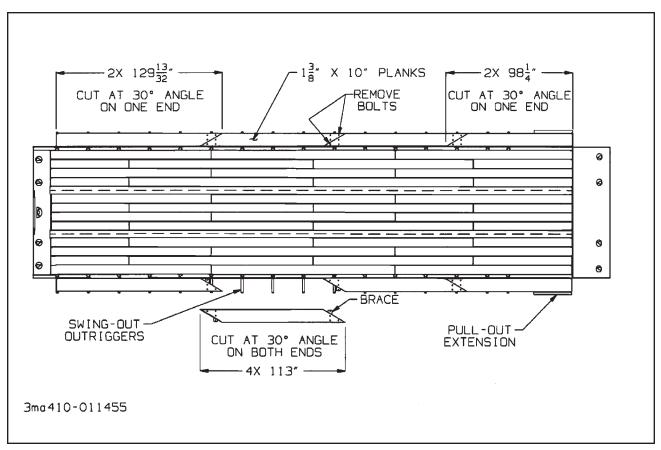
Figure 3-5 Outrigger Platform Extension
