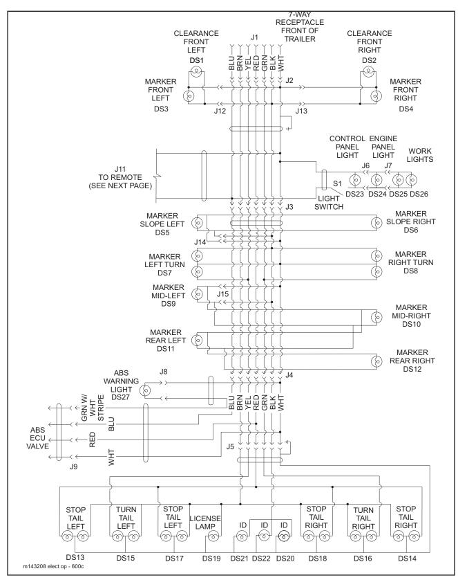
Figure 4-5 600C Wiring Diagram
