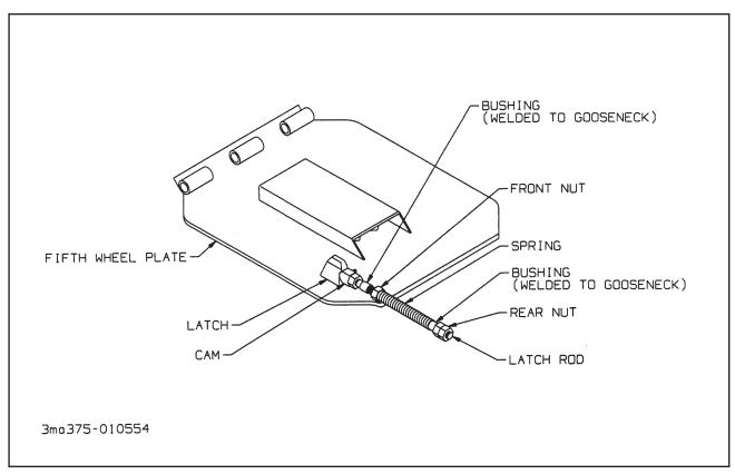
Figure 4-4 Fifth Wheel Latch Adjustment
