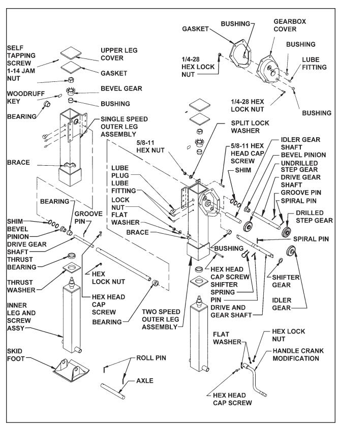
Figure 4-24 Crank Landing Gear Assembly
