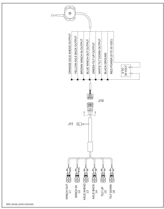
**Figure 4-6 Remote Wiring Diagram**
