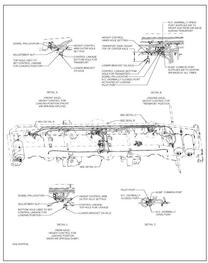
Figure 4-9 Triple Axle Air Ride Suspension System
