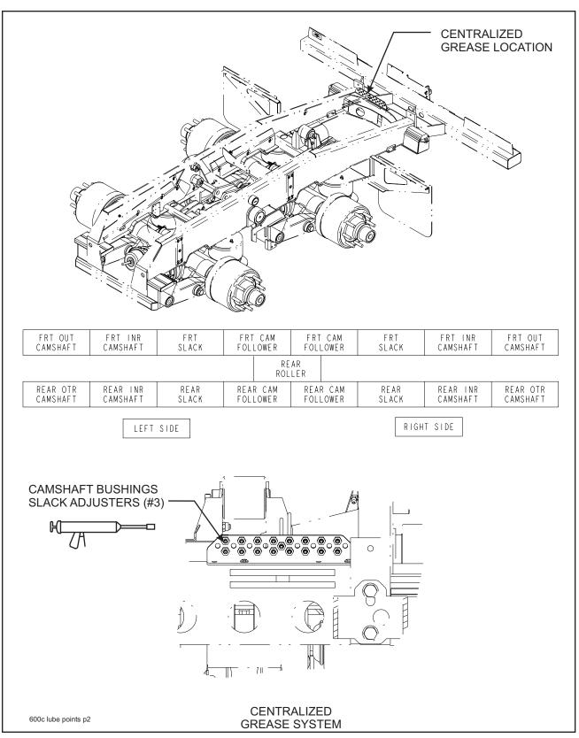
Figure 4-2 Lubrication Points (2 of 3)
