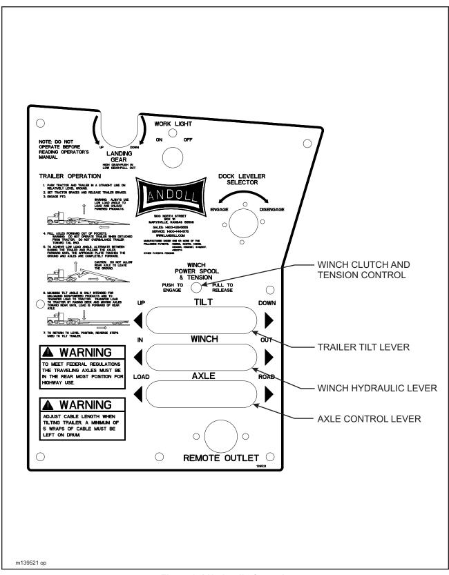
Figure 3-4 Hydraulic Controls
