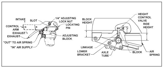
Figure 4-8 Air Ride Height Adjustment
