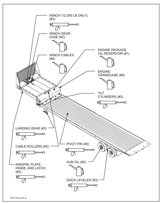
Figure 4-1 Lubrication Points (1 of 3)
