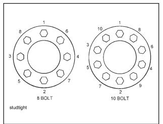
Figure 4-22 Stud Tightening Sequence
