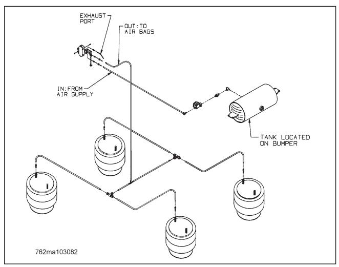
Figure 4-7 Tandem Axle Air Ride Suspension System
