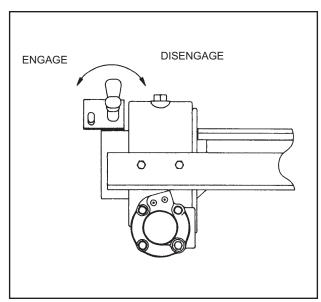
Figure 3-9 20,000# Winch Clutch
