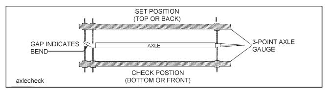
Figure 4-10 Checking Axle for Bend
