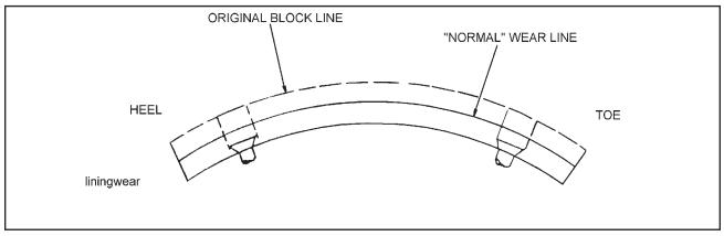
Figure 4-14 Brake Lining Wear
