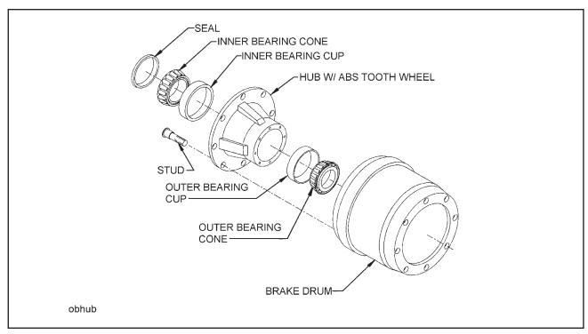
Figure 4-17 Outboard Mount Hub and Drum
