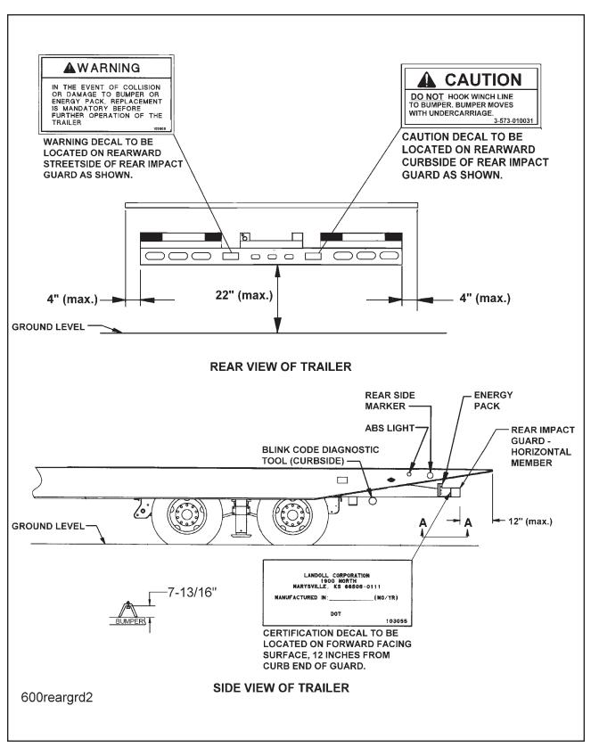
Figure 3-14 Rear Impact Guard and Antilock Brake System
