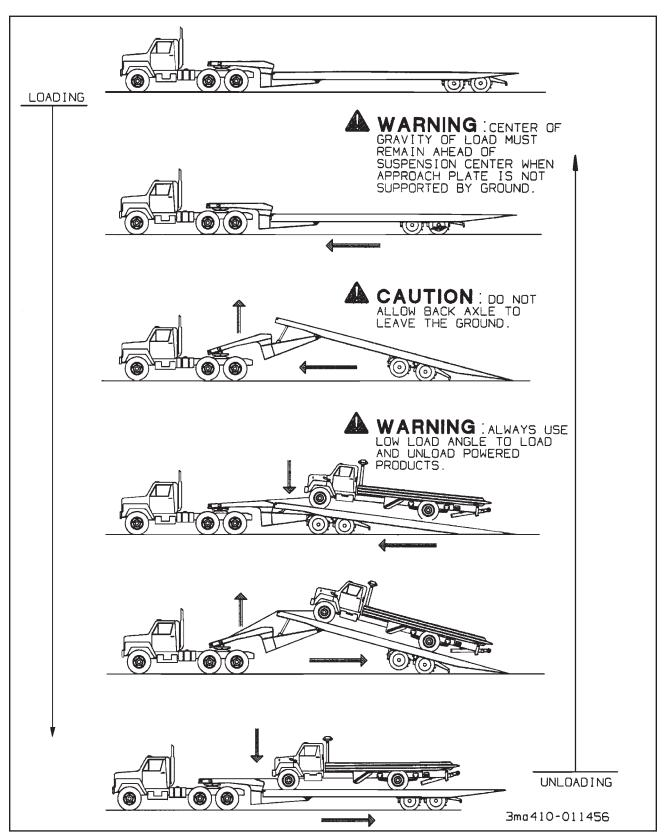
Figure 3-7 Steps for Loading and Unloading
