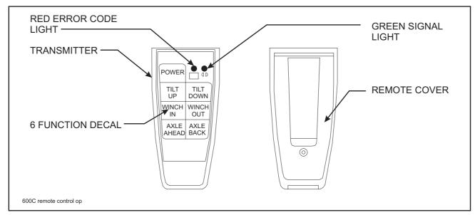
**Figure 3-13 Remote Control Transmitter**
