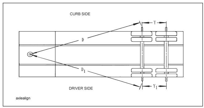
**Figure 4-11 Checking Axle Alignment**
