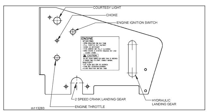
Figure 3-11 Engine Control Panel
