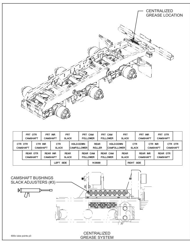
Figure 4-3 Lubrication Points (3 of 3)
