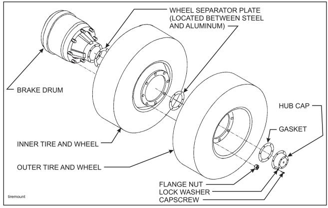
Figure 4-21 Mounting Tires and Wheels
