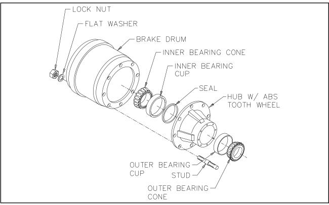
Figure 4-13 Inboard Mount Hub and Drum
