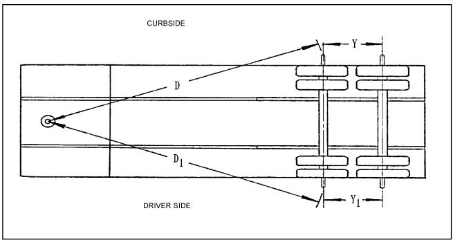
Figure 4-6 Checking Axle Alignment
