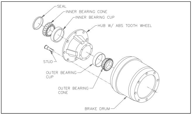
Figure 4-12 Outboard Mount Hub and Drum
