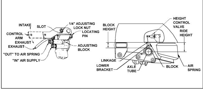
Figure 4-4 Air Ride Height Adjustment
