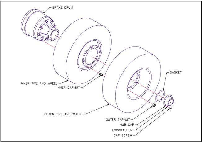
Figure 4-17 Mounting Tires and Wheels
