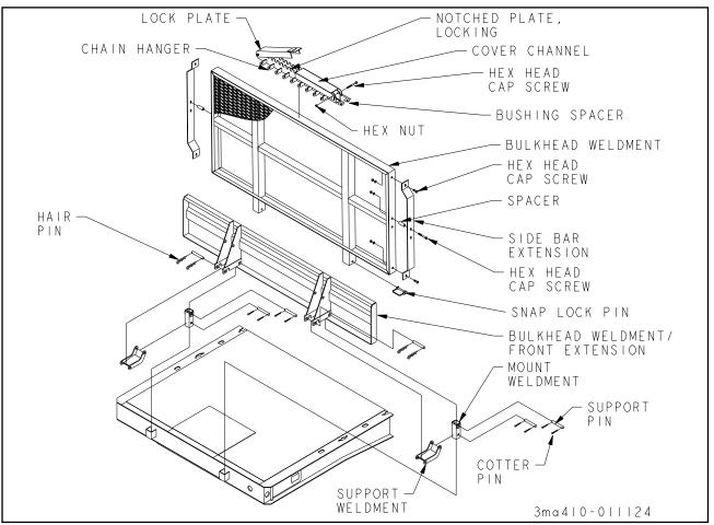
Figure 3-8 Front Extension/Bulkhead
