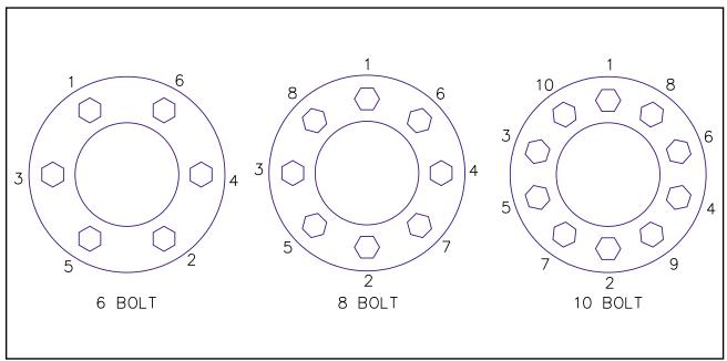
Figure 4-18 Stud Tightening Sequence
