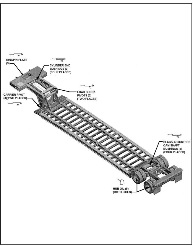
Figure 4-1 Lubrication Points
