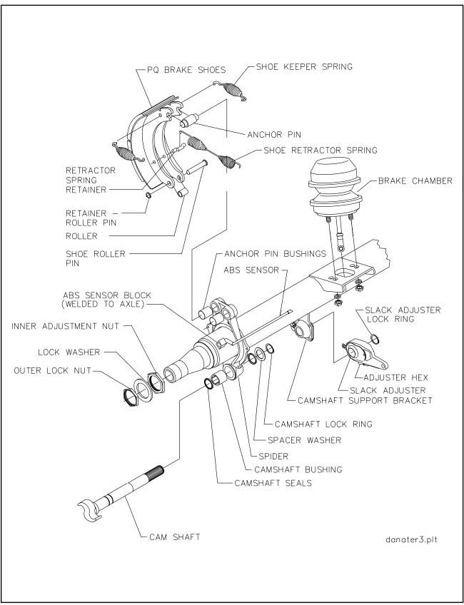
Figure 4-10 Axle and Brake Assembly
