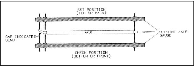
Figure 4-5 Checking Axle for Bend
