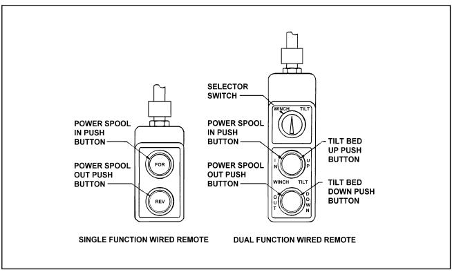
Figure 3-9 Examples of Remote Control Options
