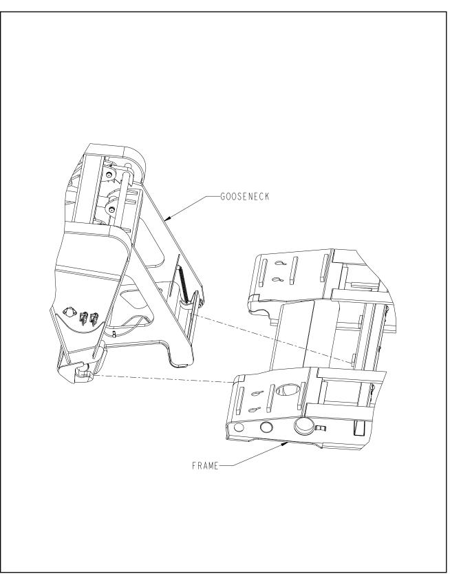
Figure 3-5 Gooseneck Attachment to Frame
