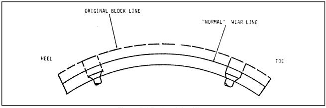
Figure 4-9 Brake Lining Wear
