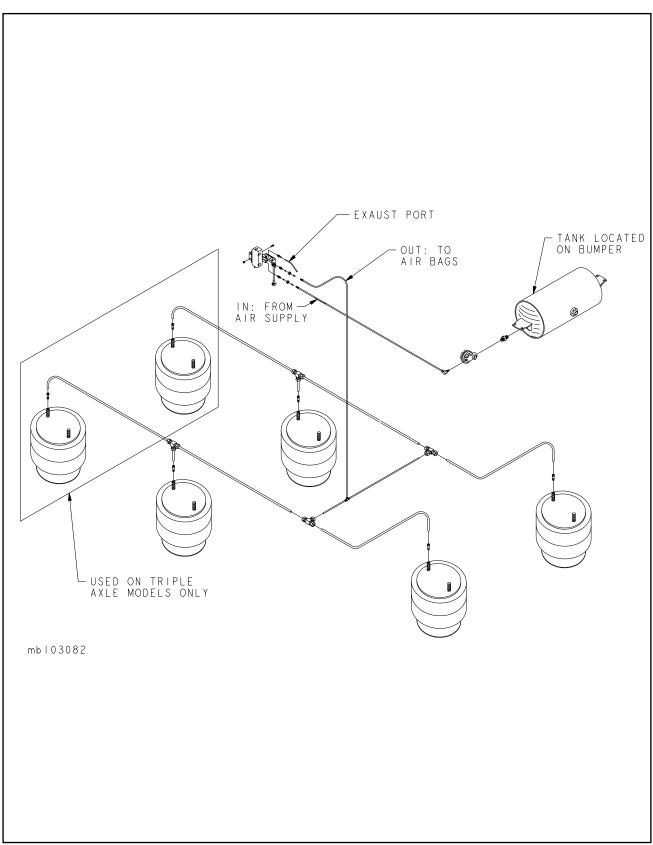
Figure 4-3 Tandem Axle Air Ride Suspension System
