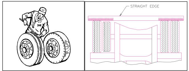
Figure 4-15 Measuring Tape Method
