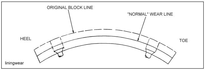
Figure 4-12 Brake Lining Wear
