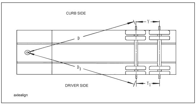
Figure 4-9 Checking Axle Alignment
