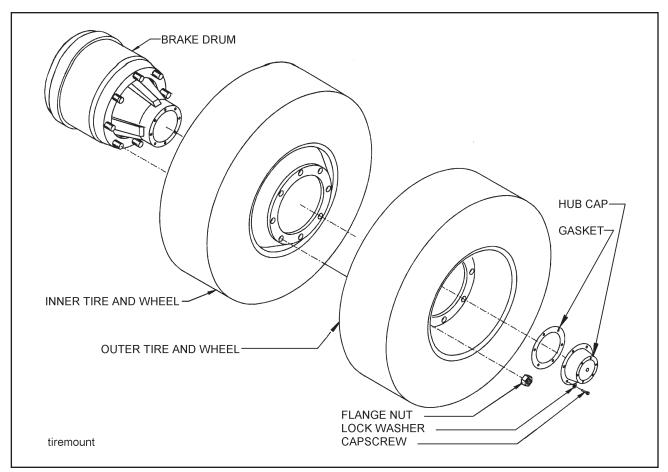
Figure 4-19 Mounting Tires and Wheels
