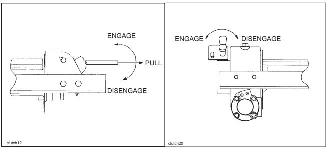
Figure 3-7 12,000# Winch Clutch
