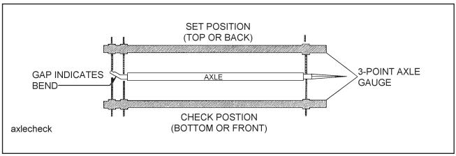
Figure 4-8 Checking Axle for Bend
