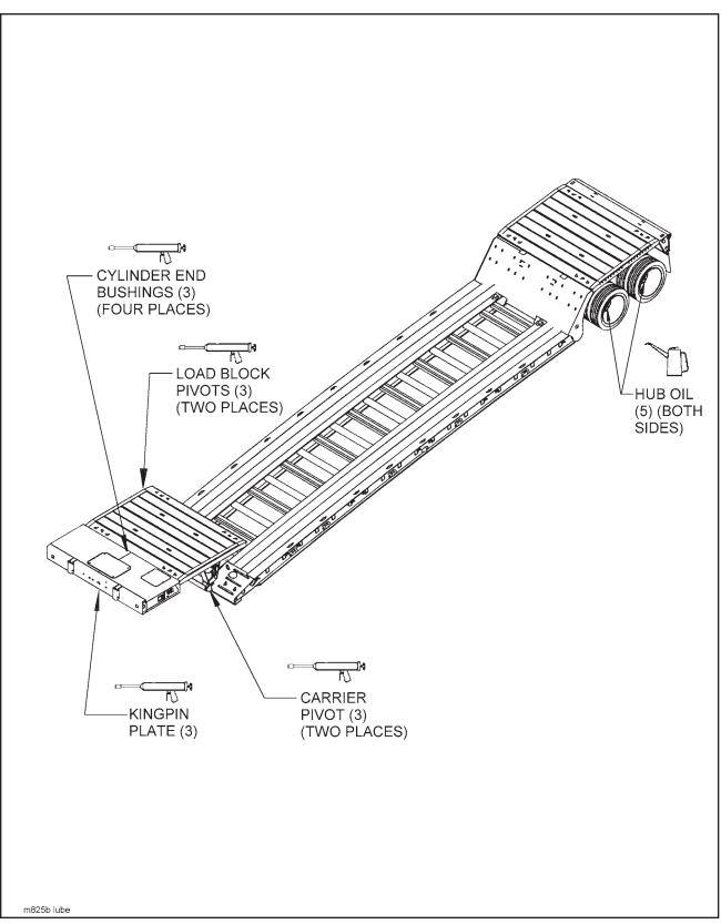
Figure 4-1 Lubrication Points (1 of 2)
