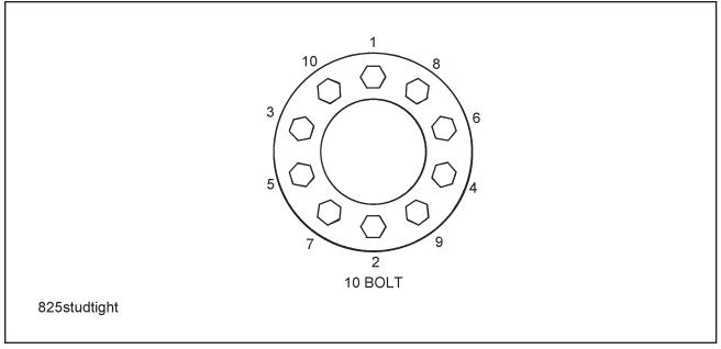
Figure 4-20 Stud Tightening Sequence
