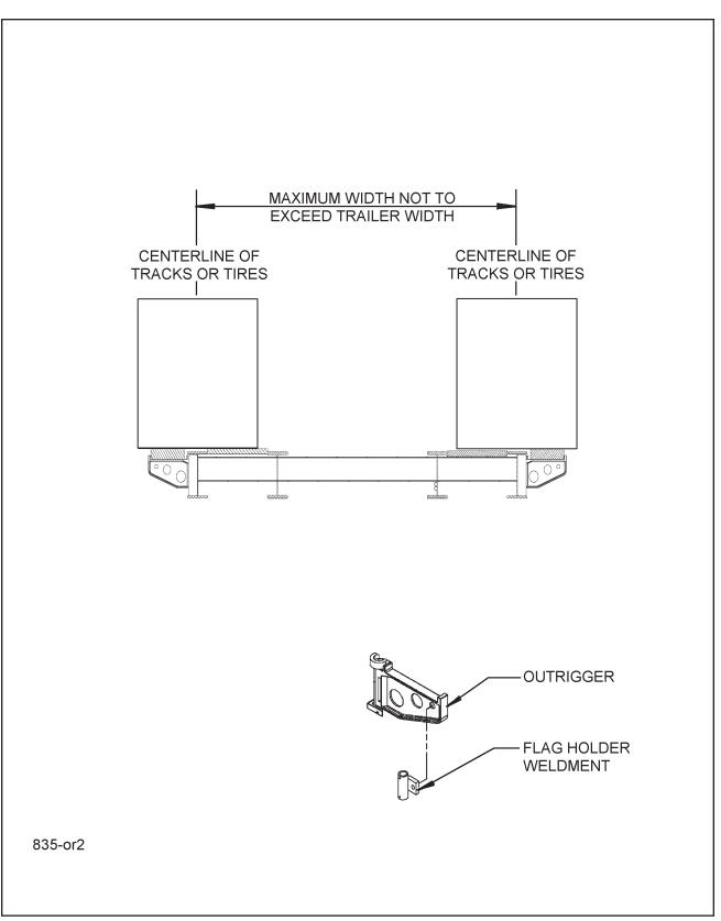
Figure 3-5 Swingout Outrigger Platform Extension
