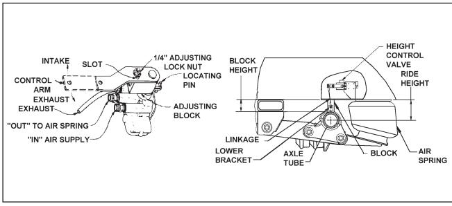
Figure 4-7 Air Ride Height Adjustment
