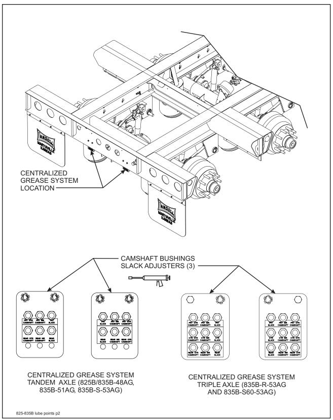
Figure 4-2 Lubrication Points (2 of 2)
