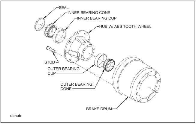
Figure 4-15 Outboard Mount Hub and Drum
