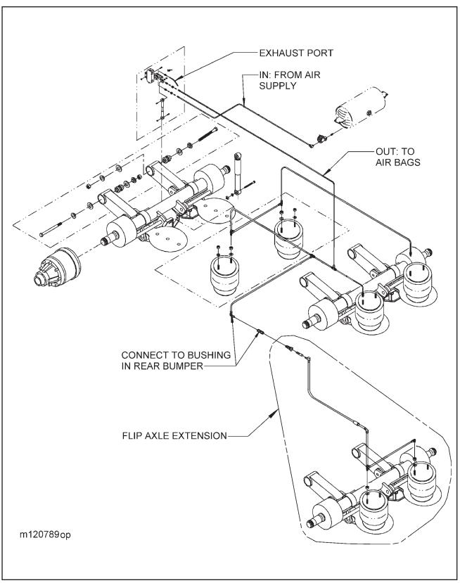
Figure 4-6 Tandem Axle W/ Flip Air Ride Suspension System
