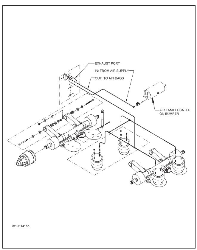
Figure 4-5 Tandem Axle Air Ride Suspension System
