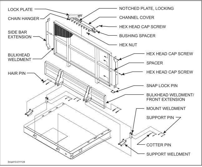
Figure 3-9 Front Extension/Bulkhead
