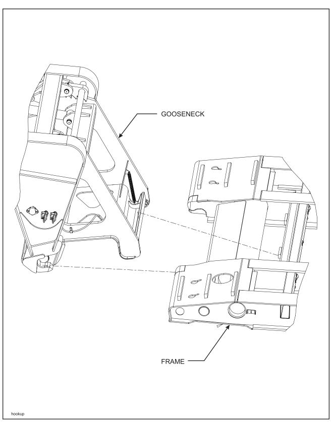
Figure 3-6 Gooseneck Attachment to Frame
