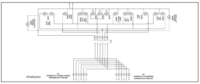
Figure 4-4 Model 835B Flip Axle Wiring Diagram
