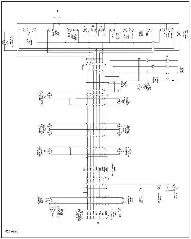
Figure 4-3 Model 825B/835B Wiring Diagram
