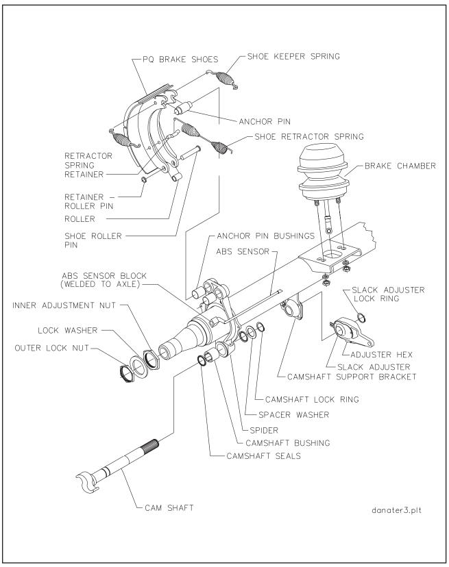
Figure 4-13 Axle and Brake Assembly
