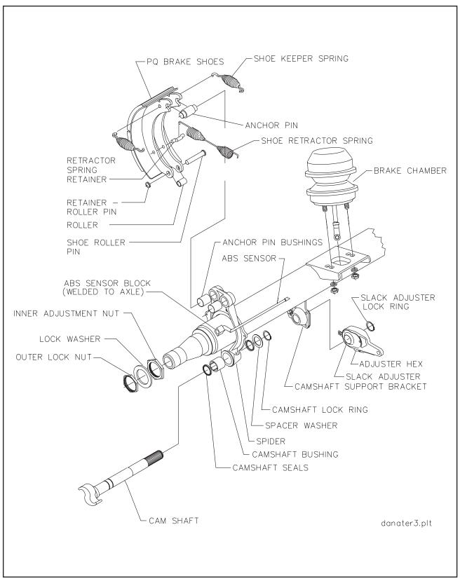
Figure 4-13 Axle and Brake Assembly
