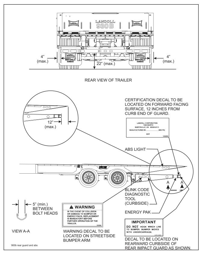
Figure 3-12 Rear Impact Guard and Anti-lock Brake System
