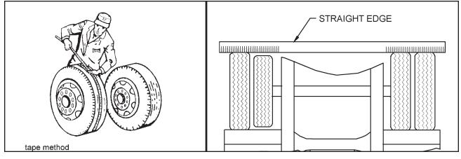
Figure 4-17 Measuring Tape Method
