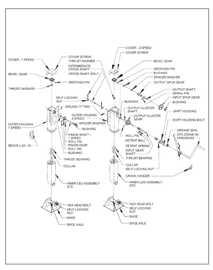
Figure 4-21 Crank Landing Gear Assembly
