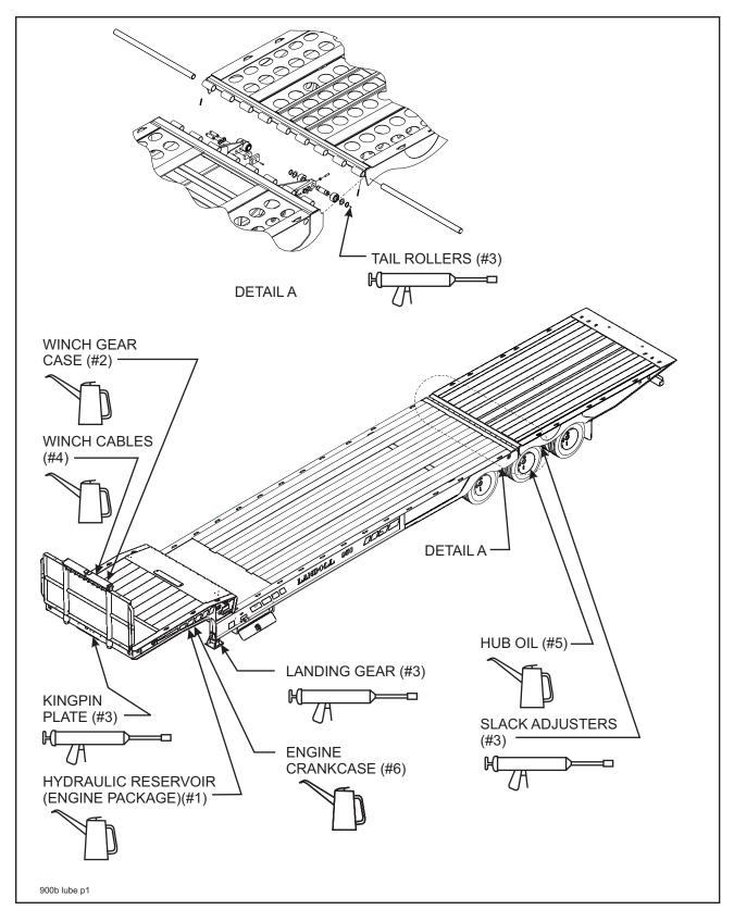
Figure 4-1 Lubrication Points (1 of 2)
