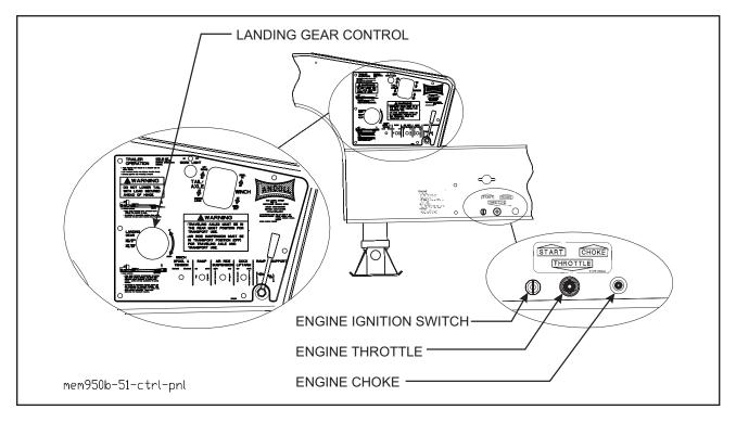
Figure 3-9 Hydraulic Engine Package Control Panel
