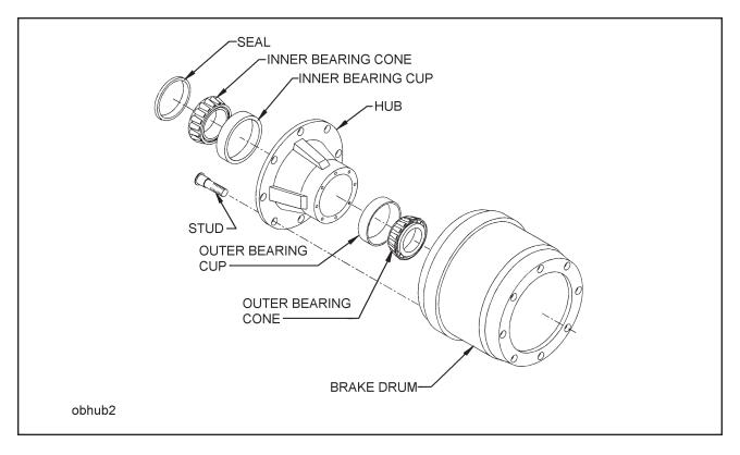
Figure 4-15 Outboard Mount Hub and Drum
