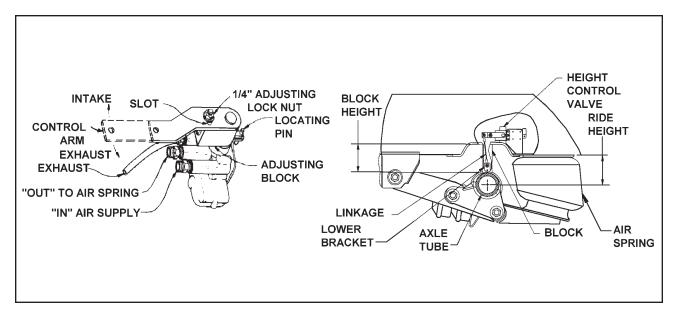
Figure 4-7 Air Ride Height Adjustment
