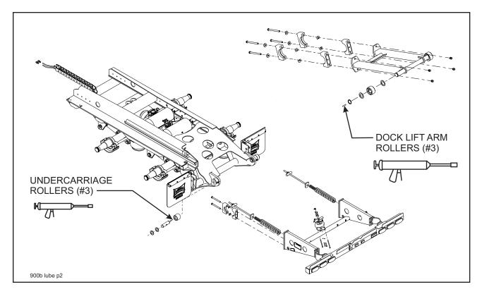
Figure 4-2 Lubrication Points (2 of 2)
