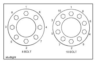
Figure 4-20 Stud Tightening Sequence
