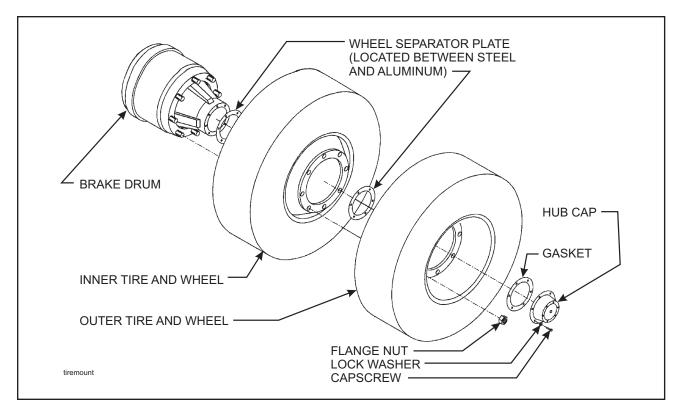
Figure 4-19 Mounting Tires and Wheels
