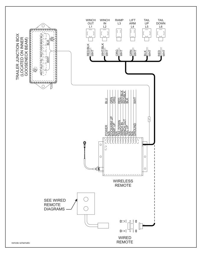
Figure 4-4 Remote Control Diagram
