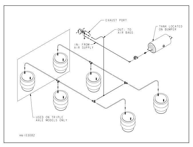
Figure 4-6 Tandem/Triple Axle Air Ride Suspension
