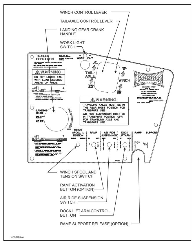
Figure 3-3 Hydraulic Controls
