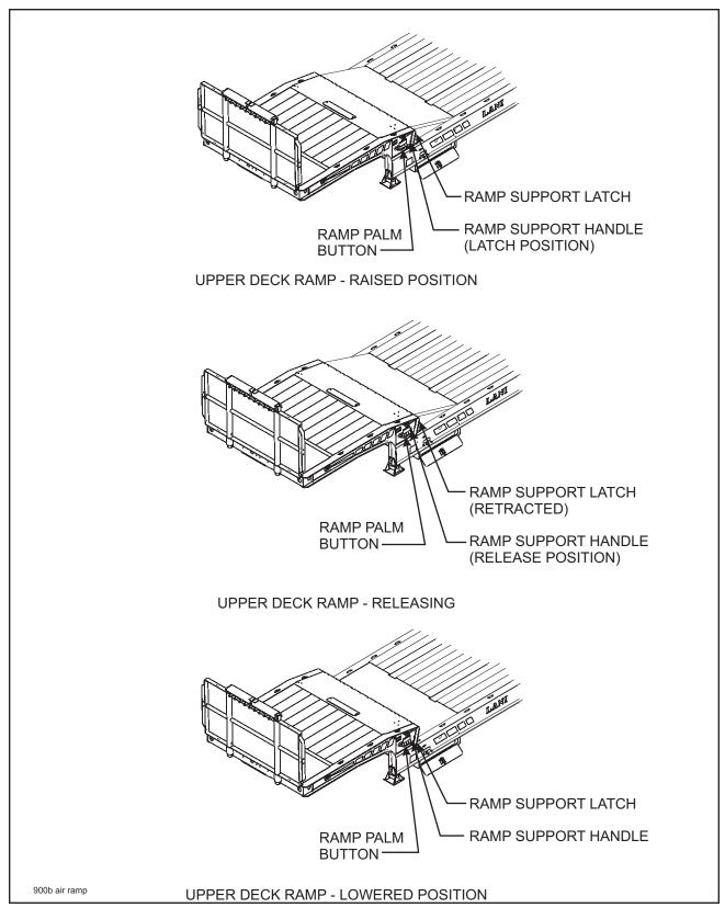
Figure 3-8 Air Activated Upper Deck Ramp (Optional)
