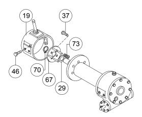
Remove two capscrews (item #46) from clutch housing (item #19) and unlatch shifter assembly.
