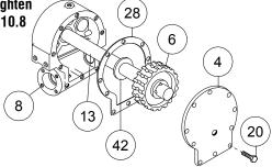
13. Press bearing (item #17) onto worm (item #14) Note: Be sure that thick shoulder of bearing's outer race (side with manufacturer's name and part number) is out, away from worm threads. Tap key (item #11) into worm. Press bearing and worm into gear housing. Slip gasket (item #27) onto bearing cap (item #2). Use four capscrews (item #20) to secure cap to gear housing. Tighten capscrews to 8 ft-lbs. (10.8 Nm) each.
