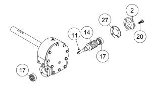
14. Press bearing (item #17) onto worm and into gear housing. Note: Be sure that thick shoulder of bearing's outer race (side with manufacturer's name and part number) is out, away from worm threads.
