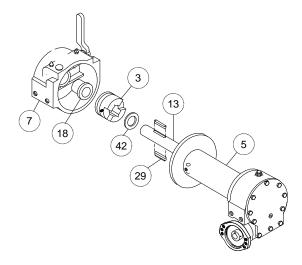
4. Remove coupling (item #25) from adapter (item #1) by unscrewing four screws (item Replace adapter seal (item #42) and gas-
