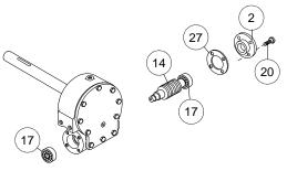
screws (item #20) to secure cap to gear housing. **Tighten capscrews to 8 ft-lbs.** (10.8 Nm) each.
