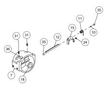
11. Check cover bushing (item #18) for signs of wear. If necessary remove old bushing and press bushing into place.
