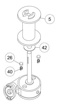
17. Place thrust washer (item #42) over end of drum shaft and slide downward until space rests on drum. Press drum downward to compress springs in gear housing.
