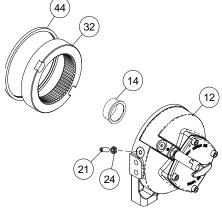
Generously apply grease (MOBILITH SHC 007) to teeth of ring gear (item #32), teeth of planet gears in drum (item #1), and to bushing (item #14) in gear housing end bearing. Apply a small amount of grease to base of bushing (item #15) on motor end bearing. Apply grease to teeth of output sun gear (item #10) and input shaft (item #13).
