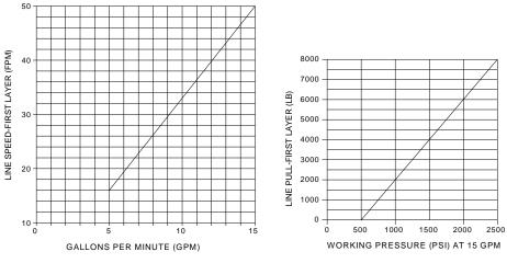
BASED ON 15.5 CU. IN. MOTOR
