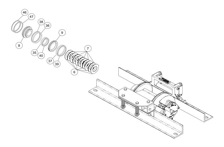
Remove nuts (item #66), washers (item #28), springs (item #60), and capscrews (item #55) from spring tensioner. Spring tensioner may be left partially assembled when removing capscrews (item #65). Refer to exploded views on pages 14 and 16 for all components. **CAUTION: Both tensioner assembly and mounting angle (item #3) will come off at the same time when mounting angle capscrews (item #65) are removed.** Slide motor end bearing (item #11) and drum (item #1) from gear housing end bearing.
