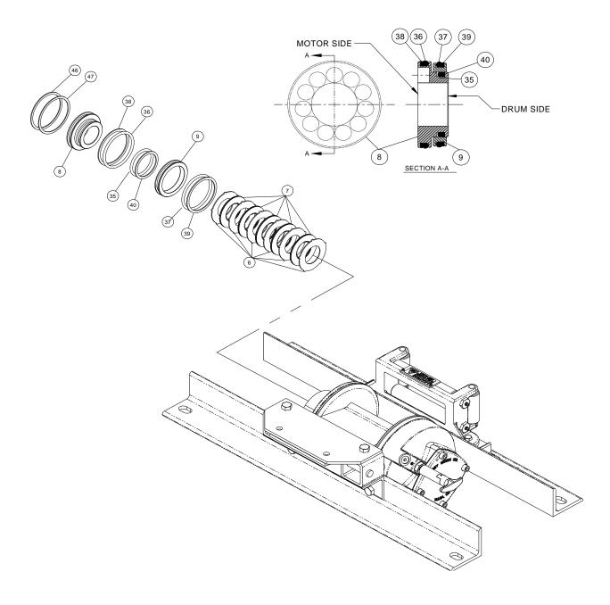
Insert springs (item #48) into pockets in back of brake piston. The two empty pockets should be on opposite sides.
