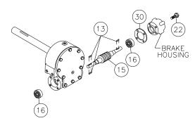
13. Press bearing #16 onto worm and into housing. NOTE: Be sure that thick shoulder of bearings outer race (side with manufacturer's name and part number) is out, away from worm threads. Place gasket #30 onto adapter #2. Attach adapter to gear housing using four (4) capscrews #23. TIGHTEN CAPSCREWS TO 12 FT. LBS. (16.3 Nm.) EACH. Insert keys #13 into keyways of worm shaft. Slide tapered end of coupling #6 over end of worm shaft. Be sure roll pin #39 is in coupling.
