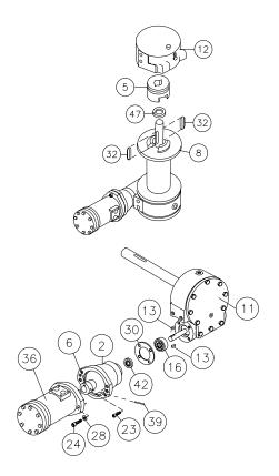
4. See page 12 for servicing the oil cooled brake. Remove brake housing mounting screws #22 and remove brake with gasket. Replace gasket #30. Remove worm #15 and bearings #16 from gear housing. Use soft hammer to gently tap input end of worm and drive worm and bearing from gear housing. Once worm has been removed from housing, bearing can be pressed from end of worm.
