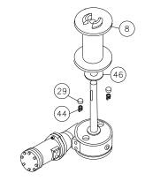
15. Place thrust washer #47 over end of drum shaft and slide downward until spacer rests on drum. Press drum downward to compress springs in gear housing.
