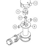
16. Attach angles #3 & #4 using six capscrews #21 with lockwashers #27 and two capscrews #20 with lockwasher #27. Torque capscrews to 34 ft. lbs. (46 Nm.) each. Insert plug #38 into bottom of gear housing. Permatex may be applied to threads to help prevent leakage.
