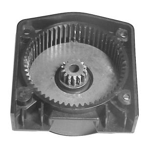
11. Re-install Carrier Assembly to Motor End Ring Gear. Twist the Carrier Assembly until the three gears fit into the Input Sun Gear underneath. When this happens, the Carrier Assembly will slide down into the Ring Gear.
