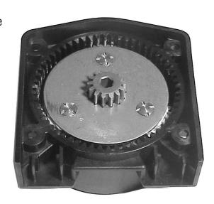
12. Re-install Thrust Washer to Ring Gear. There should be a little clearance between the Thrust Washer and the top of the gear in the Ring Gear.
