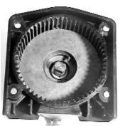
9. Insert Brake Coupling over motor shaft, as shown at right. The front tang of the spring should fit in the step in the coupling. Turn the coupling and motor shaft by hand slightly as needed to properly align the coupling with the tang.
