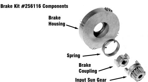
7. Slide Brake Housing into Motor End Ring Gear. If necessary, use a hammer and a large socket or short length of tubing, to drive the Brake Housing square into the Motor End Ring Gear. The Brake Housing should slide all the way into the Ring Gear.
