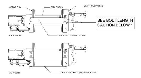
In the as-installed condition, if the winch is mid-mounted, then at least one tie-plate must be attached to the mounting feet at the bottom of the winch to maintain alignment. If the winch is foot mounted then at least one tie-plate must remain mounted at midpoint of winch to maintain alignment. It is always preferred to used BOTH tie-plates in the final installed configuration.
