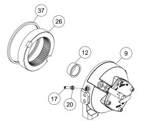
Generously apply grease (MOBILITH SHC 007) to teeth of ring gear (item #26), teeth of planet gears in drum (item #1), and to bushing (item #12) in gear housing end bearing. Apply a small amount of grease to base of bushing (item #13) on motor end bearing. Apply grease to teeth of output sun gear (item #7) and input shaft (item #10).
