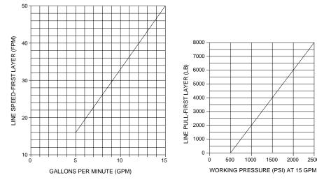
BASED ON 15.5 CU. IN. MOTOR
