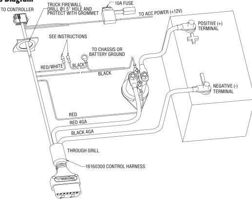
**1.** Route the CONTROL HARNESS through the truck grill, by the battery, and through the firewall. Some trucks will require drilling a ø1.50" hole through the firewall, while some will have holes provided (usually plugged). Check your truck Owner's Manual for details. If the hole is drilled it is critical that a grommet be used to prevent damage to the wire harness.
