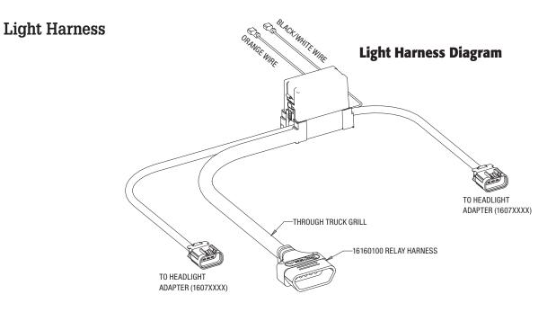
**1.** Route the RELAY HARNESS through the grill (drivers side preferably) and place the RELAY MODULE close to either the drivers or passenger side headlight (whichever is convenient).
