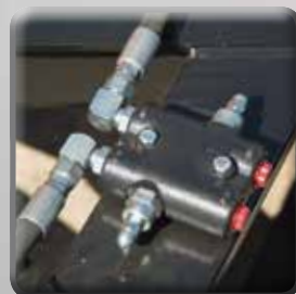
⑮ 10 GPM cushion valve with 1/2" ports protects cylinders from impact loads. Preset at 2000 PSI, adj. from 1500 - 3000 PSI
