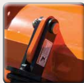
⑤ 3-position attack angle for adjustable trip of 5°, 10°, or 20°
