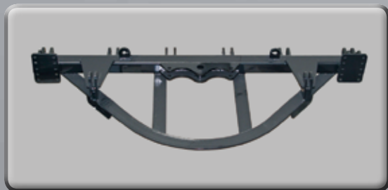
⑯ 80" Semi-circle has 3-1/2" x 3-1/2" x 1/2" angle, welded to the 3-1/2" x 3-1/2" x 5/16" structural push tube 90" wide
