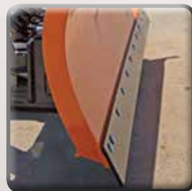
⑩ 1/2" x 6" standard one piece carbon steel cutting edge (highway punch)
