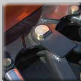
⑭ 3-1/2" steel channel A-frame supports a 1-1/2" plated king pin mounted in a 2-1/4" OD x 3/8" wall DOM tube, with grease fitting
