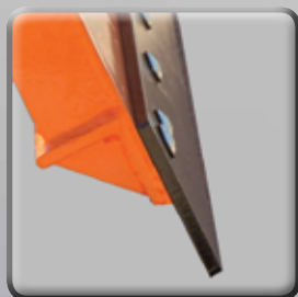
⑪ Reinforced 3-1/2" x 3-1/2" x 1/2" bottom angle with 1/2" reinforcement gussets every 12"
