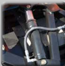
⑬ Twin 3" single acting chrome plated hydraulic cylinders for heavy duty power reversing. Located above the push frame for protection & ease of service
