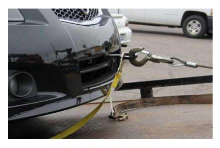
**I-Bolt** is a 2ö x 1 ½ö loop connected to a 7ö long steel shaft with unique gripping teeth that lock into the threaded holes on the front or rear of the vehicle. Insert the **I-Bolt** into the threaded hole, ideally behind the nut or the back of the hole, engage the gripping teeth by turning the loop clockwise (while holding the knurled 1 ¾ö knob) until the teeth engage behind the nut or in the threaded hole.
