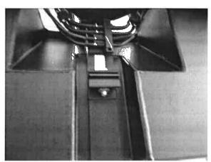
31. Make sure that the tank is not touching the frame rail, if it is you will need to push the tank to the driveshaft side as much as possible. Torque the frame rail nuts to 32 ft-lb  $\pm$  2 ft-lb then torque the driveshaft side bolts to 32 ft-lb  $\pm$  2 ft-lb.
