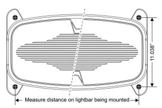
Caution: Permanent mounting of this product will require drilling. It is absolutely necessary to make sure that no other vehicle components could be damaged by this process. Check both sides of the mounting surface before starting. If damage is likely, select a different mounting location.
