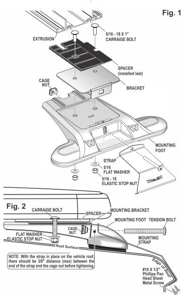
Slide the bracket to the outer end of the base extrusion and secure the bracket to the extrusion by tightening the elastic stop nuts. Repeat steps 1 - 3 for other side of lightbar.
