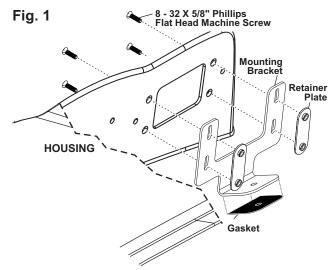
IMPORTANT! The lightbar should be a minimum of 16" from any radio antennas! NOTE: A Mid Roof Transit is shown in this installation for example. The High Roof Transit mounts the same.
