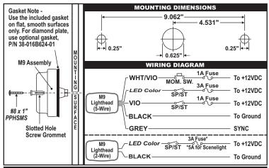
Waterproof butt splices and/or connectors are required if that connection could be exposed to moisture. Any unused wires must be sealed (waterproofed) to prevent moisture infiltration.
