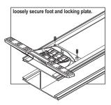
NOTE: Model MKAJ is an adjustable mounting foot. On this model you may loosen the screws on the rear of the foot and adjust the angle of the lightbar. This feature can be used if the angle of the roof is not level with the road.
