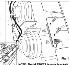
NOTE: Model RBKT1 (single bracket) is shown for example. Model RBKT2 (double bracket), mounts the same way.
