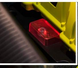
GreenFully ChargedRedChargingAmberFault DetectionBlueForeign Object Detection
