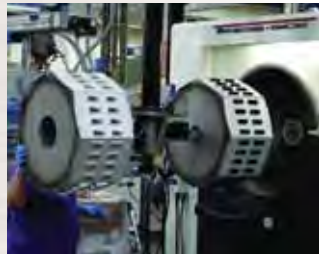
5 Vacuum Metallizing Reflector Machines
