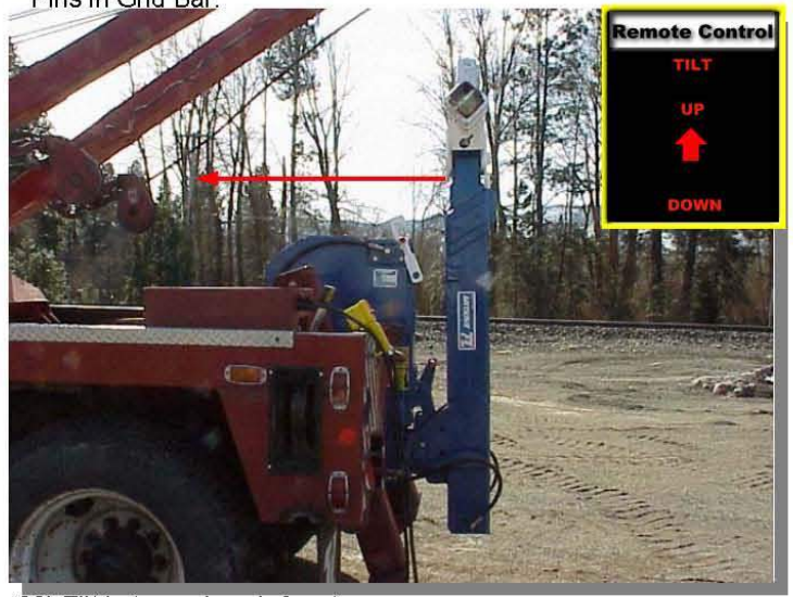
29) Tilt in towards cab for storage.
