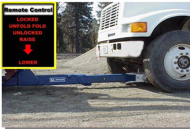
22) Lower Horizontal Extend Tube to clear undercarriage obstructions and low air foile before retracting.
