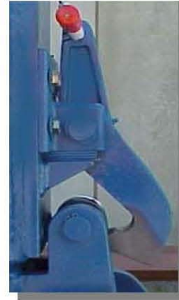
19) UNLOCK J Lock by pushing in towards main body.
