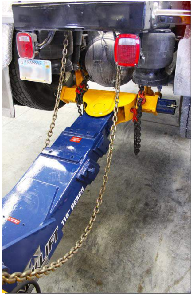
#12) Secure load to towing vehicle with Safety Chains. Failure to secure vehicle in tow voids warranty.
