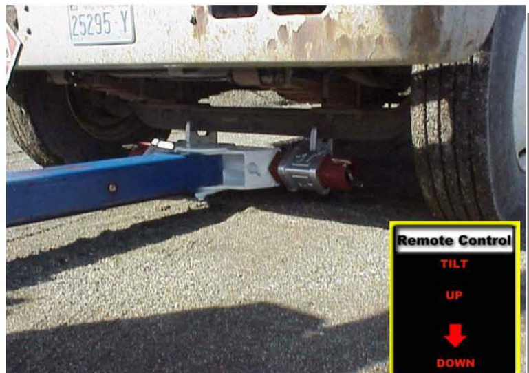
21) TILT down until tires touch the ground.
