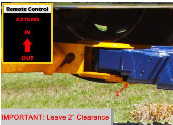
#11) Z403/Z303: Extend middle horizontal extend tube at least 2" from outer horizontal extend tube. This will create an equalization of pressure with inner tube, allowing head to pivot properly during towing. The head will appear to be locked against the inner extend tube but will disengage when turning.
