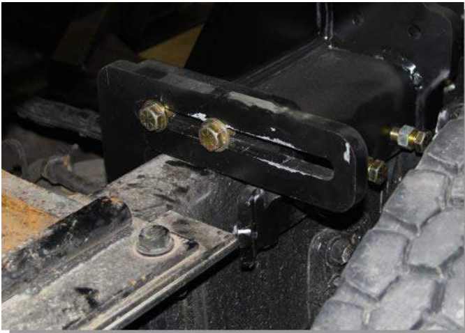
#13) Use frame clamp to secure FIFTHWHEELER foot to truck frame.
