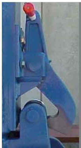
5) Unlock J Lock by pushing in towards vertical tube. May have to raise to clear J lock pin.
