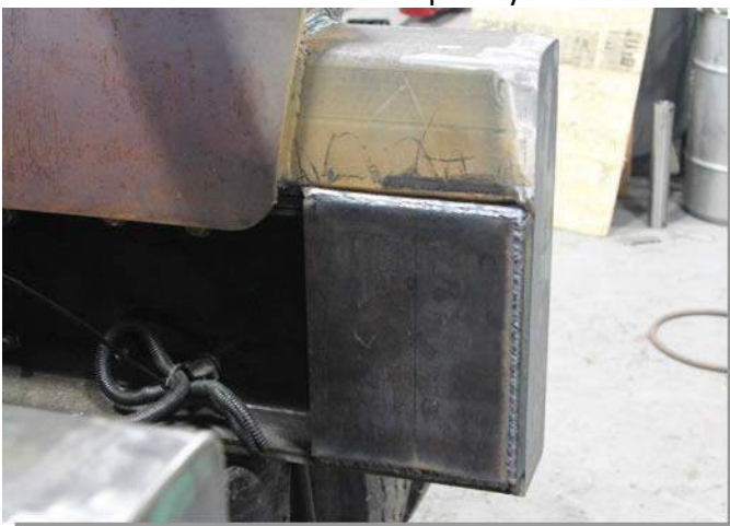
#17) Use 1/2" plate to box the end of subframe and truck frame. Enclose the truck frame at least 10 to 12 inches from the end.
