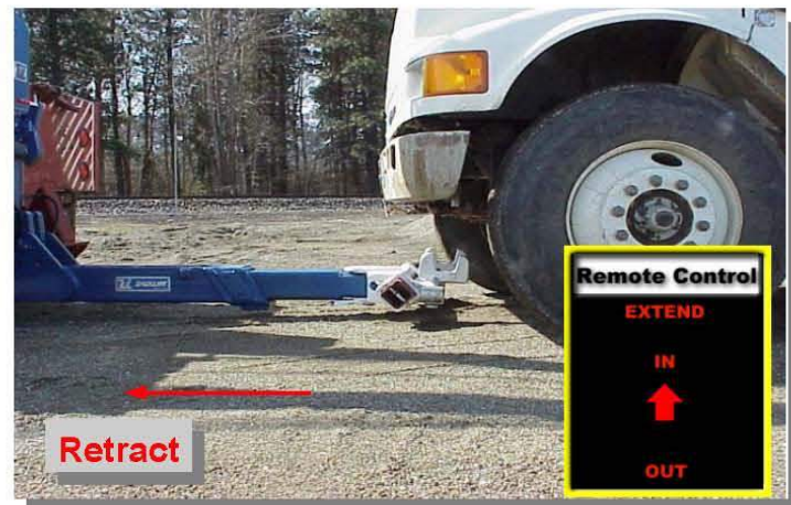
23) RETRACT (Extend In) Horizontal Extend Tube to locking position to avoid pivoting when in storage position.
