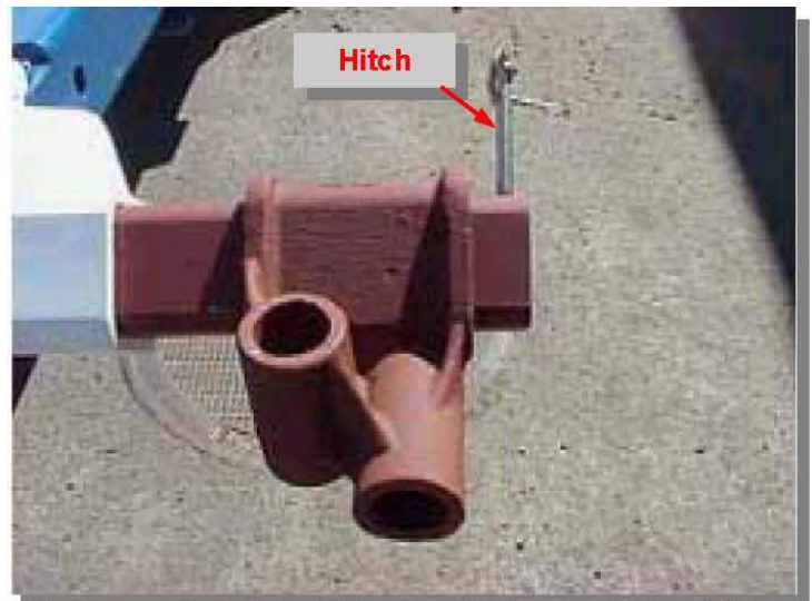
27) Remove Forks & Fork Brackets for storage. Replace Hitch Pins in Grid Bar.
