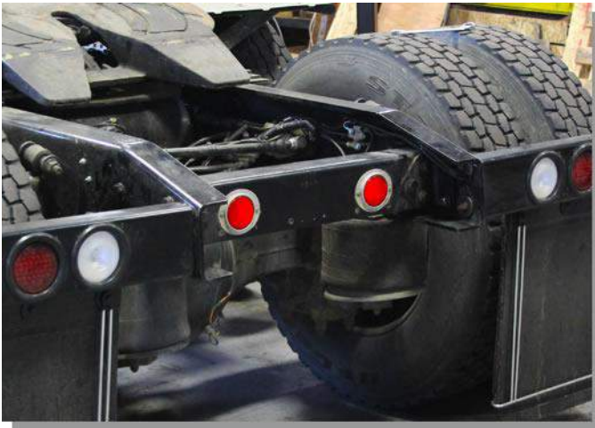
#1) Begin by removing rear crossmember. Remove all mounting brackets and electrical wiring from the rear. Retain bolts for reuse.
