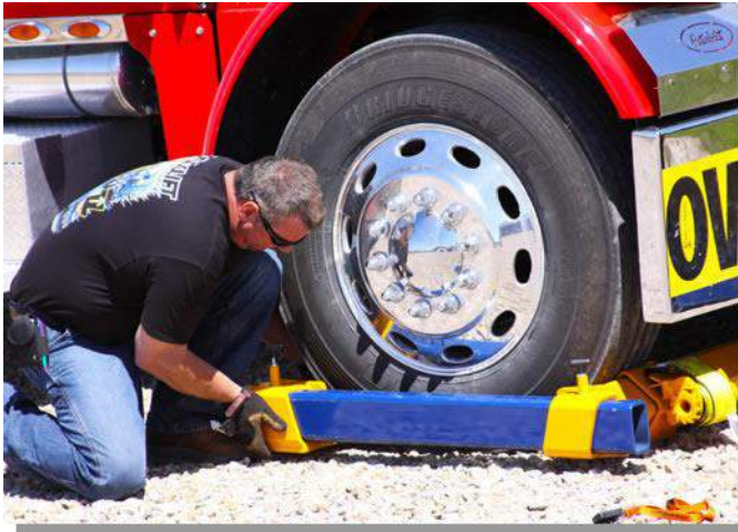
#7) Slide wheel tray onto wheel rod and against tire. Make sure pull pins are both fully engaged.
