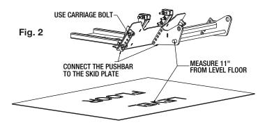
**5.** Torque all fasteners as shown in the chart. Check and re-torque all fasteners after 5 hours of usage to ensure safe plow operation.
