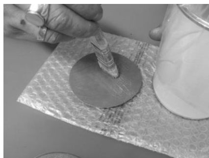
Fig. 6: Glue application. Glue SC-2000 is black colour.
