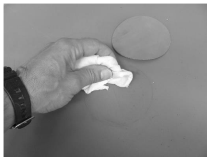
Fig. 5: Cleaning of the glued area.
