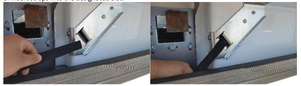
4. Pro tip: jam the straps into the lower corner of the slot to ensure the straps do not come out. Then, drop and center SpaceKap onto truck.
