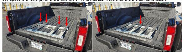
If your truck is one of the models below, you need to install the provided round rubber bumpers and hardware to the closed end of the C channels that do not already have them fastened in order shim the overall length of the install kit. They go in the square hole closest to the bend.
