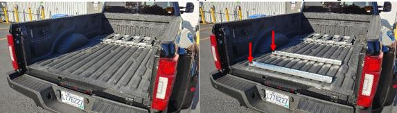
11. Take the four (4) remaining **C** channels **with** the round rubber bumpers and place them on top of the A crossmembers. The **closed end** of the C channels with the rubber bumpers must be **towards the rear**.
