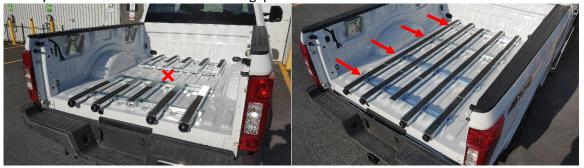
17. <u>FOR 6.5' AND 8' BED</u> – Use all four (4) **E** channels to link the front section to the rear section.
