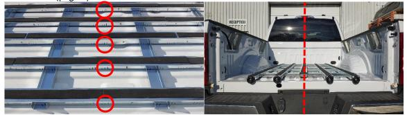
22. <u>FOR AN 8' BED</u> – Ensure the **double** arrows at the end of the **E** and **F** channels sit **into** the A crossmember of the front section of the kit using the **same** height setting as the front and rear sections. Please note these channels are **wider** than the C and D channels and will **overlap** them.
