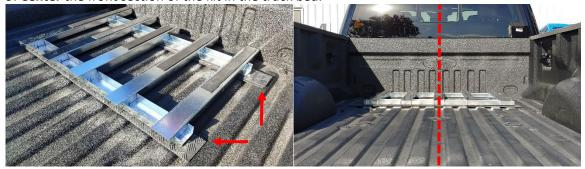
10. Back at the rear of the truck bed, place two (2) A crossmembers on top of the grooves.
