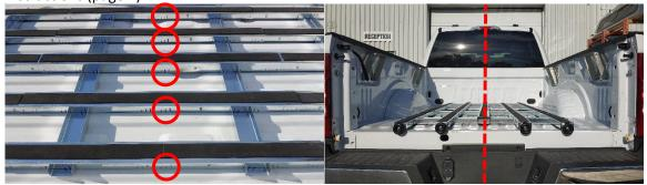
22. <u>FOR AN 8' BED</u> – Ensure the **double** arrows at the end of the **E** and **F** channels sit **into** the B crossmember of the front section of the kit using the **same** height setting as the front and rear sections. Please note these channels are **wider** than the C and D channels and will **overlap** them.
