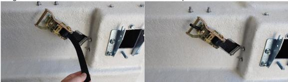
8. The SpaceKap should now sit closer to the bed railings, 1/8" to 1/2" is the preferred gap. To finish the installation completely, cap off the holes with provided brackets and hardware.
