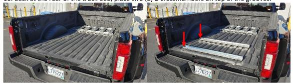
11. Take the four (4) remaining **C** channels **with** the round rubber bumpers and place them on top of the B crossmembers. The **closed end** of the C channels with the rubber bumpers must be **towards the rear**.
