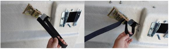
7. Tighten the ratchet buckles lightly at first beginning with the front and finishing with the rear. Once all four have some tension you can tighten them as much as you can. Doing it this way will prevent the SpaceKap from shifting as you apply pressure. Push the excess of the strap into the designated slot and secure the ratchet buckles with a tie-wrap.
