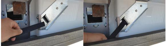
4. Pro tip: jam the straps into the lower corner of the slot to ensure the straps do not come out. Then, drop and center SpaceKap onto truck.
