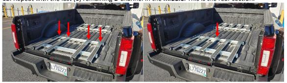
13. Ensure the height setting is the same for **all** the C and D channels and that it matches with the front section.
