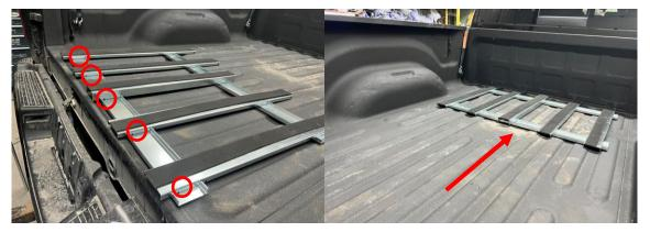
9. Back at the rear of the truck bed, place two (2) **192 (42",one notch)** crossmembers on top of the grooves.
