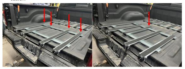
12. Ensure the height **setting #1** is the same for **all** the **193** and **194** channels and that it matches with the front section.
