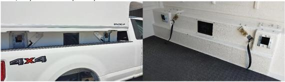
5. Ensure the SpaceKap sits level from side to side. If it is crooked, some components of the install kit might not be in their intended position. A difference of an eighth of an inch (1/8") is acceptable. The SpaceKap should not sit higher than an inch (1") from the truck's bed rails.
