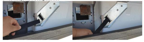
4. Pro tip: jam the straps into the lower corner of the slot to ensure the straps do not come out. Then, drop and center SpaceKap onto truck.
