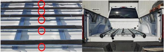
21. <u>FOR AN 8' BED</u> – Ensure the **double** arrows at the end of the <u>195 (42",two notch</u>) and <u>196 (42",two notch and tall)</u> channels sit **into** the <u>192 (42",one notch</u>) crossmember of the front section of the kit using the **same** height setting as the front and rear sections. Please note these channels are **wider** than will sit on top.
