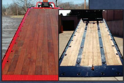
Century's 20 & 30 Series decks are available with an optional Apitong wood floor in place of the standard diamond steel floor plate. The black carrier bed pictured includes the optional dual key slots down the center of the floor, as well as key slots and lashing rings along the deck edge.
