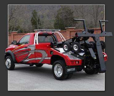
With increased rear visibility, positive and negative power tilt with limiter switches, a low profile crossbar with recessed pins and redesigned jaws, the operator can quickly and easily hook up to most vehicles from the safety and comfort of the cab of the truck.
