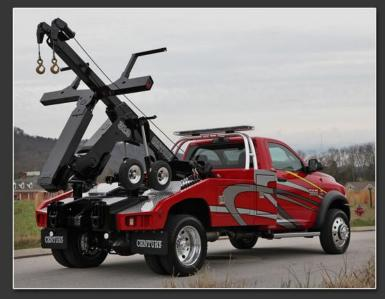
The Century Express Gen II features a hydraulic extendable recovery boom, twin lift cylinders, single or dual 8,000 lb. winches, along with passenger and driver side manual control stations provide the operator with recovery capabilities not usually found in most auto-load units.
