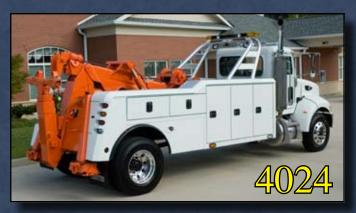
The 4024/T2 with over 102" of reach on the underlift is ideally suited to handle a wide variety of vehicles such as motor homes, delivery vans, and city tractors. This single axle unit with a 20-ton recovery boom and 20,000 lb. winches creates an incredible value with features only found on larger units.
