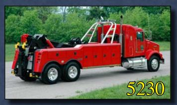
The 5230 is designed to be the ideal unit for towing when scale weight is an issue. The 5230 provides 113" of underlift reach to easily handle most vehicles and is standard with Century's weight-saving aluminum body. A 30-ton recovery boom and 25,000 lb. winches completes this popular package.
