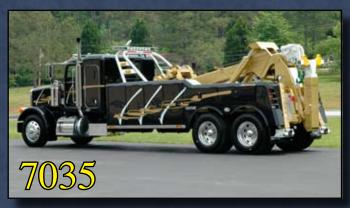
The 7035 is Century's most popular heavy-duty unit. The underlift provides 129" of reach and is designed to scale in most situations. The 35-Ton recovery boom and dual 35,000 lb. winches allows the 7035 to tackle the toughest lifting and recovery jobs, making it extremely versatile for heavy-duty towing and recovery.
