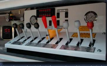
Manual controls, winch air-free spools, and 2-speed winch switches are standard on drivers & passenger side control stations. The rear switch panel is standard on the 7035 & 9055 and is available with the Power Touch System on the 4024, 5130, and 5230. The Engine Data Information Center is available as an option to monitor vital engine readings.
