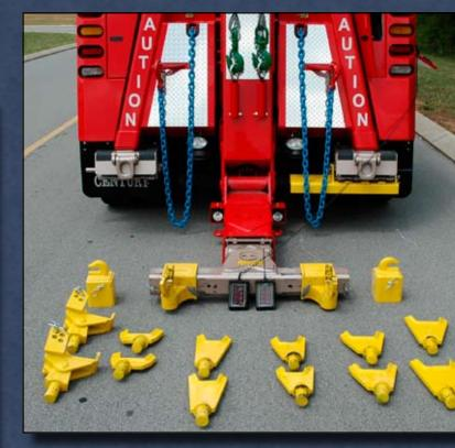
Standard equipment includes lanyard remote control, along with wide variety of lifting attachments. The 7035 & 9055 also include wireless remote as standard equipment.
