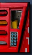
The rear taillight compartments on the aluminum body provide quick access to a pair of lifting forks and safety chains, along with the optional tailboard underlift controls.
