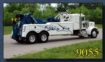
The 9055 is Century's largest capacity integrated towing and recovery unit. With a 50-ton recovery boom, with an optional third stage, and dual 50,000 lb. winches, the 9055 is ideal for heavy recovery work along with the ability to tow a wide variety of vehicles from mixers and packers through buses with its 136" of underlift reach.
