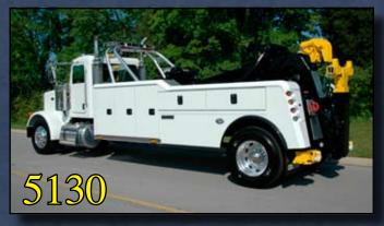
The 5130 is Century's Largest single axle integrated towing and recovery unit with 113" of underlift reach. The 5130 has the ability to tow most vehicles without giving up maneuverability of a single axle unit. The 5130 also provides a 25-Ton recovery boom and 25,000 lb. winches for your recovery and lifting applications.
