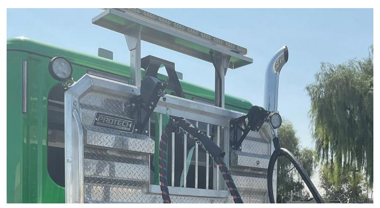
Shown above. Headache rack with 25 lb. tensioner mounted on driver's side with 3-in-1 wrapped hoses and 40 lb. tensioner mounted on passenger side with two hydraulic hoses.
