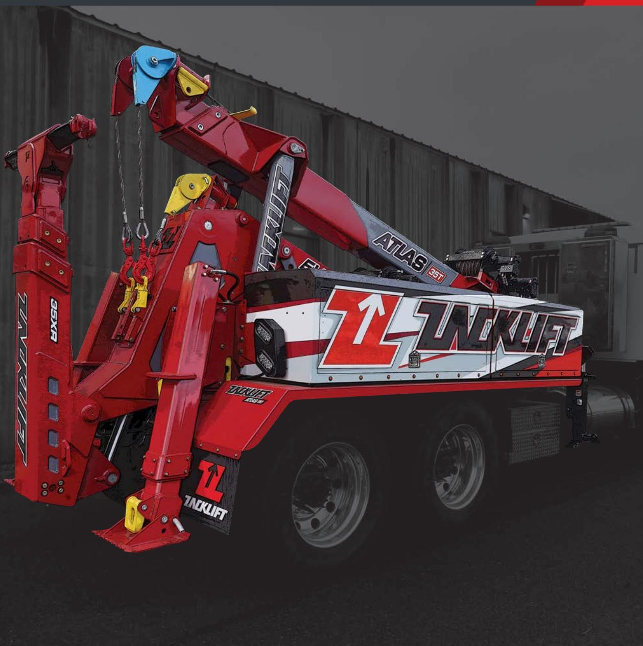
The Zacklift ATLAS 35T represents the next evolution in detachable towing technology – a purpose-built, **independent 35-ton boom** system featuring our **patent-pending EVO 35K underlift**.
