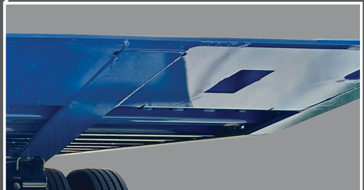
• Enclosed Approach Design to Prevent Collecting Dirt and Rocks
