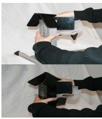
(4). While securely holding the front-stop channel in one hand, carefully use your other hand to lift the lower portion of the cradle out and away from the v-bracket which is attached to the front-stop channel
