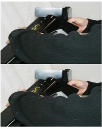
(3). Using both hands, carefully raise the front stop channel and cradle together to an upright position.
