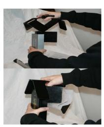
(5).Once you have cleared the lower portion of the front-stop v-bracket with the cradle, you can now lift the cradle straight up and away from the entire unit.
