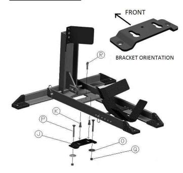
**Step 1**: Attach Shoulder Screws (K) to the Condor® Pit-Stop/Trailer-Stop cross member as shown. (Torque parts K to 18 ft-lbs)
