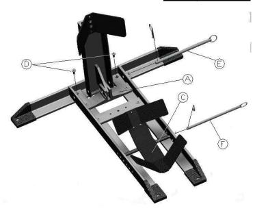
Step1: Using screws (D), attach the Base Bar (B) to the Main Unit (A). (3/16 allen wrench required, torque between 16 - 18 ft-lbs)
