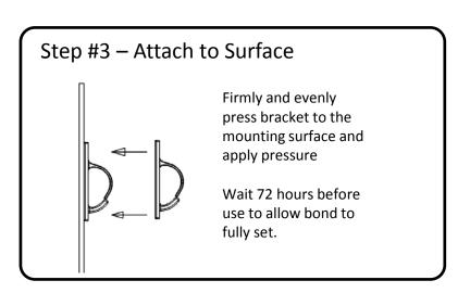
NOTE: Mounting surfaces must be free of dirt, oils and grease. Surfaces must be flat and smooth and free of voids or protrusions for maximum performance.
