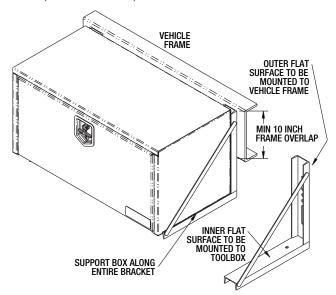
Additional fabrication may be necessary to complete this installation. Buyers Products Co. recommends contacting a qualified and trained truck equipment dealer for installation. Install fasteners with threadlocker adhesive and follow the manufacturer instructions for its application.
