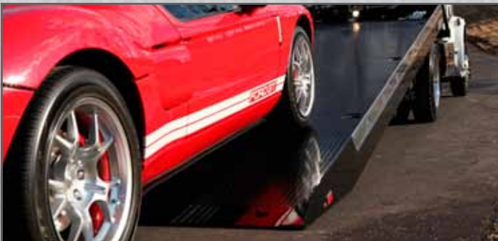
The SST™ option, available on the steel LCG™ with removable side rails or the aluminum LCG™ with solid narrow aluminum side rails, reduces your load angle by an additional 3 1/2 degrees.
