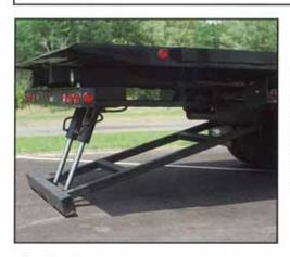
The optional hydraulic dock stabilizer provides for quick and easy loading from docks. The full width tail light housing encloses the wiring for longer
