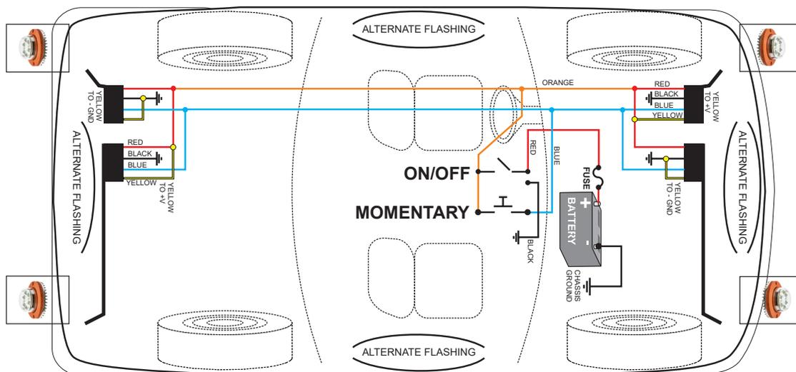
The front and rear heads are configured to flash independently of each other. In order to have the front and rear heads flash in synchronization, the blue wires from all units must be connected. The yellow wire can then be used to determine either alternate or simultaneous flash between each unit in the system by connecting to either power or ground.
