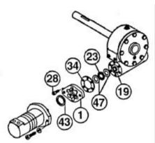
5. Remove bearing cap (item #4) from gear housing by unscrewing six capscrews (item #26). Remove worm (item #19) and bearing (item #22)
