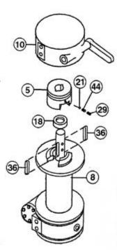
hole in jaw clutch as a guide, to drill a 1/8" deep detent (as measured to the center of the drill point) in shaft. Slide jaw clutch upward 15/16" and drill second detent.
