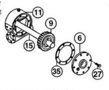
7. Check gear teeth for signs of wear. Replace if necessary by pressing gear (item #9) from shaft. Press new gear over shaft and keys until end of keys, on long end of shaft, are flush with gear. Examine shaft, keys and keyways. If distortion of keys and/or keyways are evident, shaft and keys should be replaced. Tap keys (item #14) into shaft keyways. Press gear over shaft and keys until end of keys, on long end of shaft, are flush with gear.
