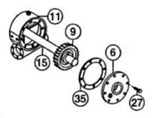
Press bearing (item) #22) onto worm (item #19). NOTE: Be sure that thick shoulder of bearings outer race (side with manufacturer's name and part number) is out, away from worm threads. Press bearing and worm into gear housing. Slip gasket (item #34) onto bearing cap (item #4). Use six capscrews (item #26) and lockwashers (item #33) to secure cap to gear housing. Tighten capscrews to 12 ft. lbs. (16.1.Nm.) each.
