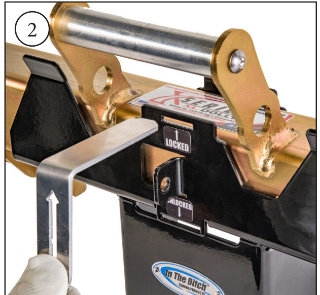
2 Remove the locking pin when ready to use the dolly.
